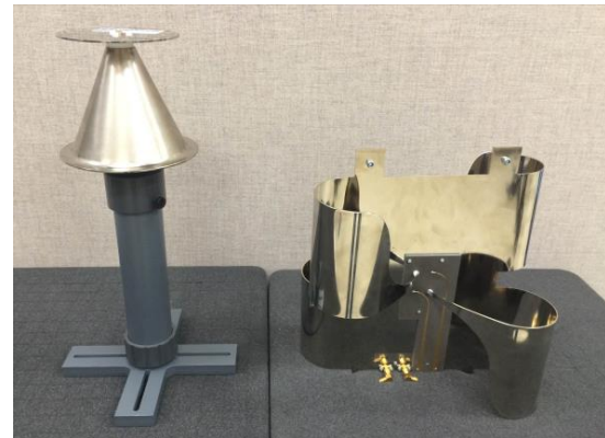
Fig. 3. Two transmit antennas; left: vertically-polarized broadband discone monopole antenna; right: polarization-balanced, double-sided, tapered, self-grounded monopole antenna [25].
