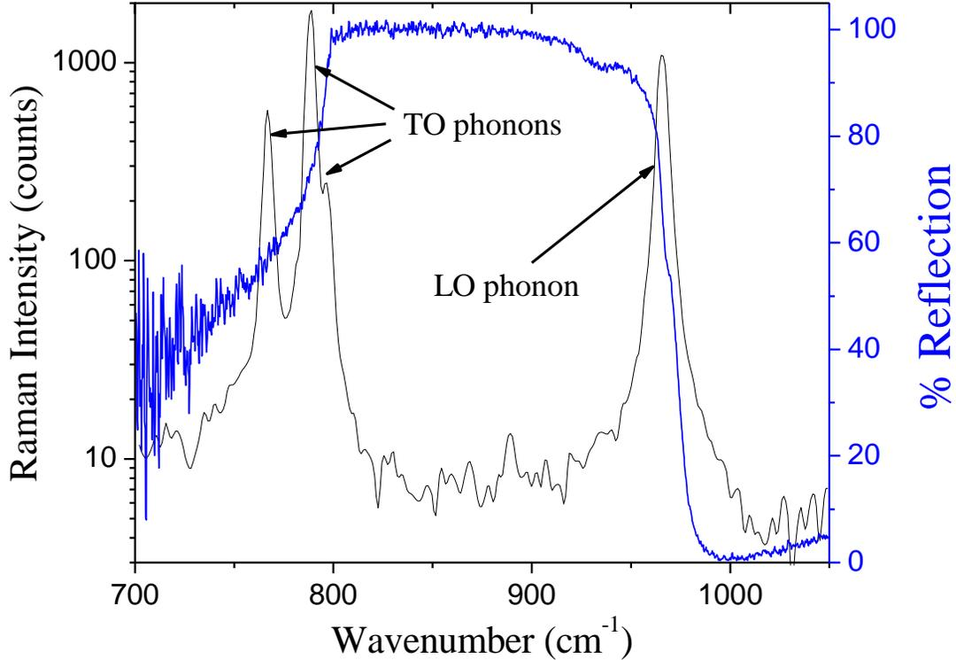
**Figure 1:** Raman spectra (black line) and reflection spectra (blue line) of un-patterned 6H-SiC. The phonon resonances are seen in the labeled Raman peaks which bound the highly reflective Reststrahlen band.
