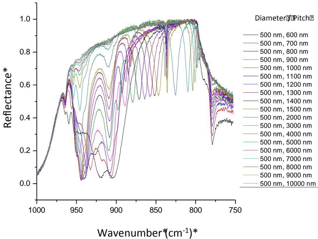
**Figure 3:** SPhP resonances in nanopillar arrays of 500 nm diameter SiC pillars. By varying the center to center distance (pitch) of the pillars in these arrays, one can precisely tune the spectral positions of these absorptive resonances.
