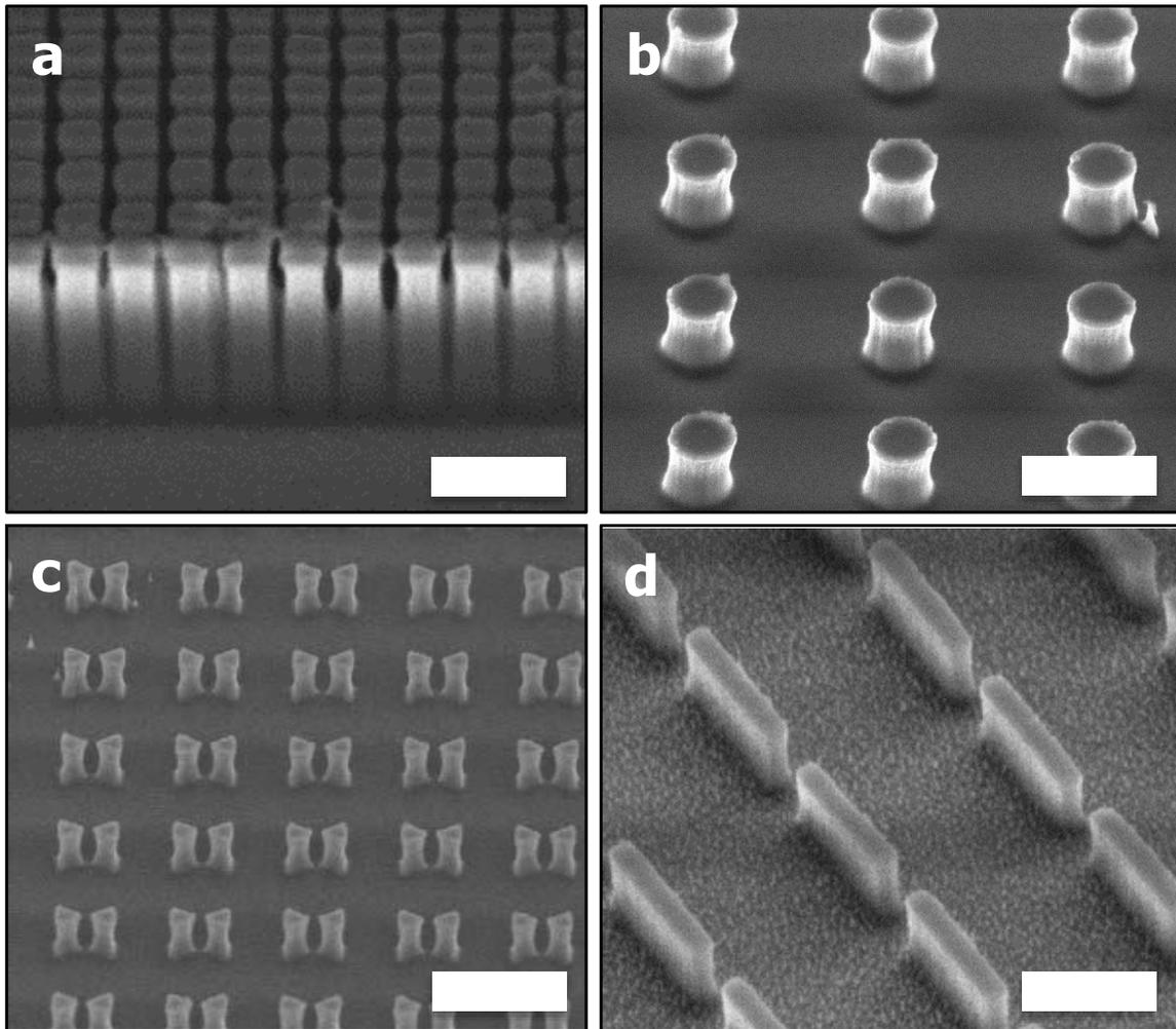
**Figure 2:** Different designs of phonon polariton nanoantennas fabricated in SiC. All scale bars are 1000 nm. **a** Closely spaced nanopillar array. **b** Widely spaced nanopillar array. **c** Coupled bowties. **d** High aspect ratio cuboids.
