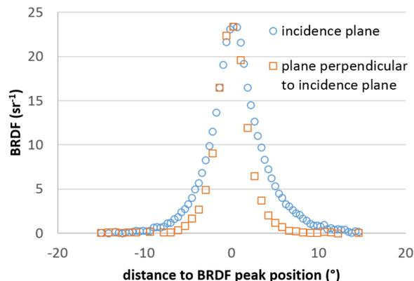
**Figure 4.** Three dimensional measurement of the BRDF of the NIST-SG#7 sample (left) for an incidence angle of 60°. Comparison between the BRDF profiles of the NIST-SG#7 sample extracted from the three dimensional measurement in the incidence plane and perpendicular to the incidence plane (right).
