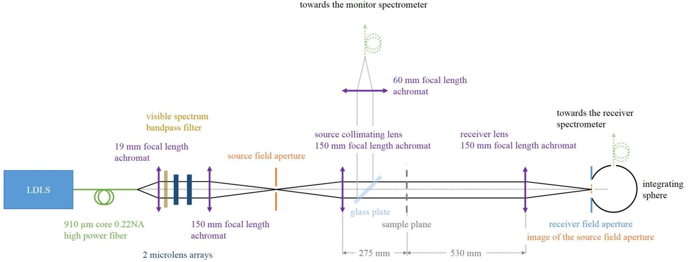
**Figure 2.** Diagram of the proposed optical system to measure gloss on the Five-Axis Goniometer. Note that distances are not to scale on the diagram. The distance between the two lenses surrounding the two microlens arrays is about 15 mm and the distance between the two microlens arrays is equal to the focal lens of the microlenses (5.1 mm).
