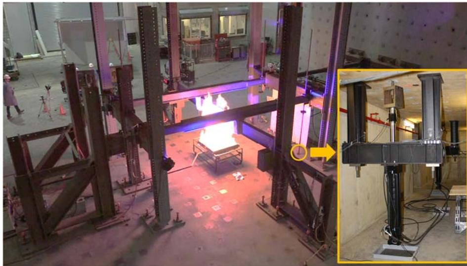
*Figure 3 NFRL commissioning test setup and structural loading system*
