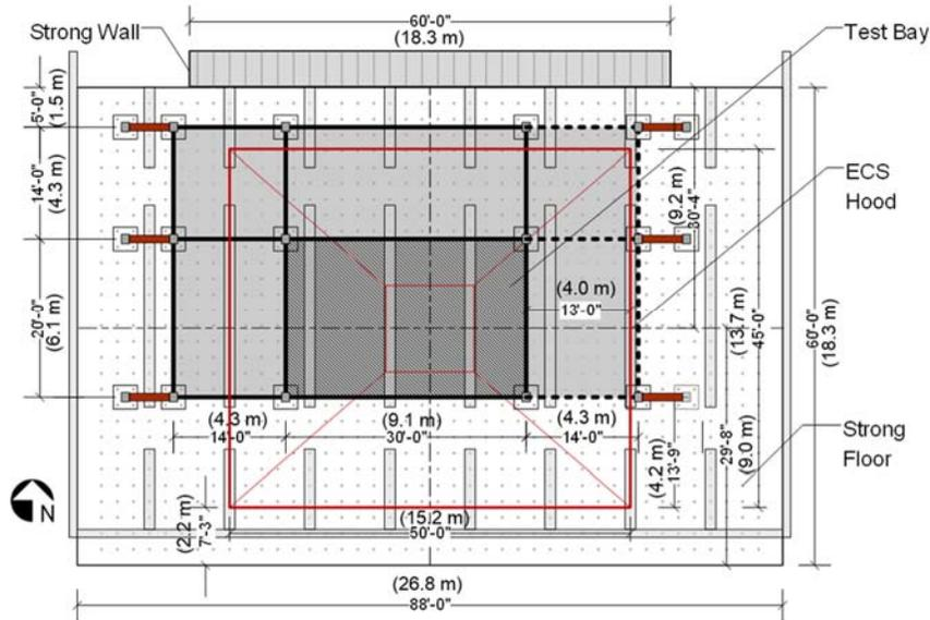
Figure 6 General plan view of test frame on the strong floor
