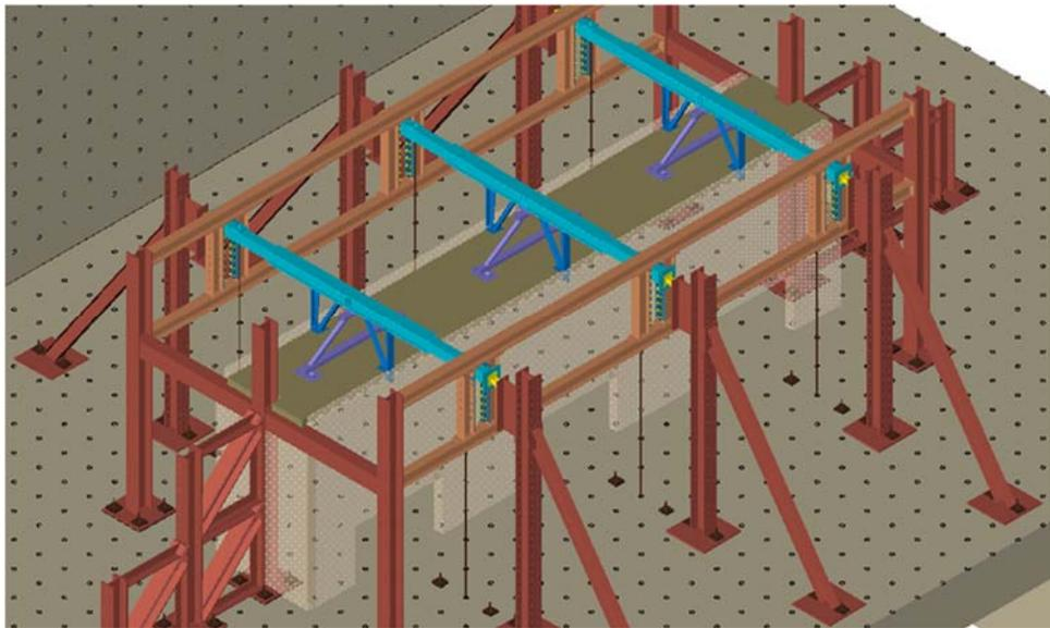
*Figure 5 Schematic of long-span composite beam test setup*
