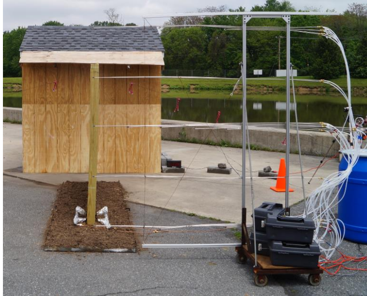
Fig. 2. Experimental setup from point between fan and fence, showing position of bidirectional probe array.
