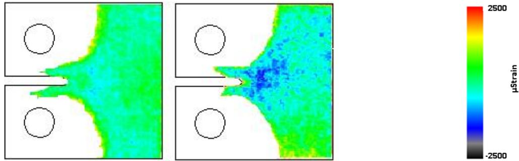
**Figure 1: Measured elastic strain fields for the cracks grown in air (left) and in H<sub>2</sub> (right). The strain direction measured is in the direction of the through-thickness of the CT specimen. The tensile applied load at the pinholes lead to tensile in-plane strains at the crack tip, which give rise to the compressive strain field in the through-thickness direction, as presented here.**
