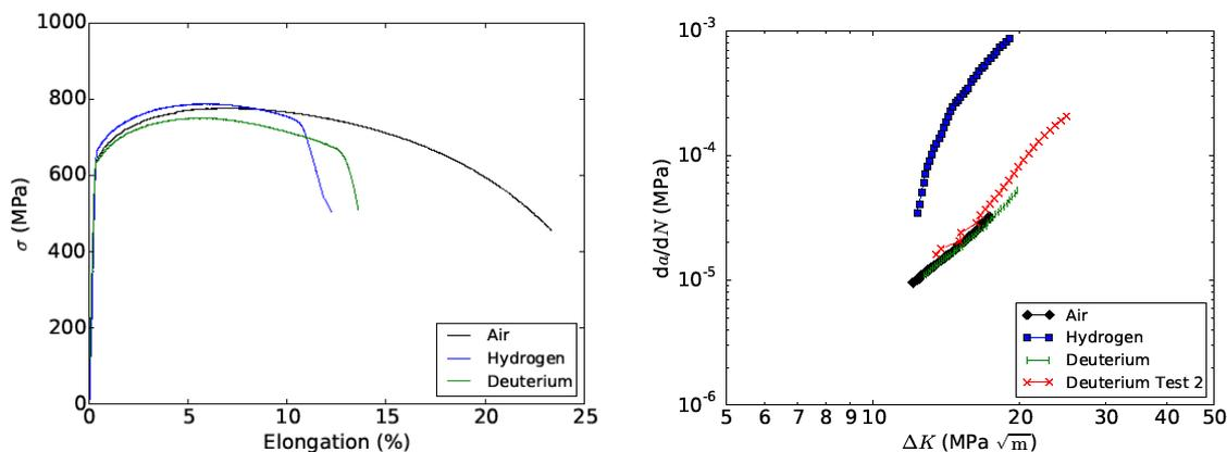
**Figure 2: Stress-strain curves for steel specimens measured in air, hydrogen, and deuterium (left). Both hydrogen and deuterium present an embrittlement effect as compared to air, indicated by a decrease in the elongation to failure. Fatigue data in the three environments (right) show a strong hydrogen assisted FCGR as compared to air, with negligible deuterium assisted FCGR.**
