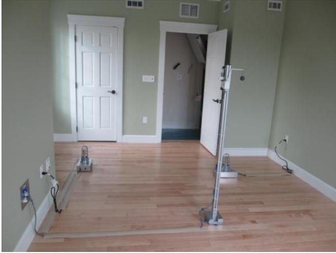
Figure 5: Thermal comfort sensors and simulated loads in a bedroom.
