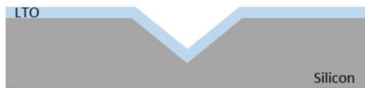
3) Silicon Oxide stripping and LTO deposition
