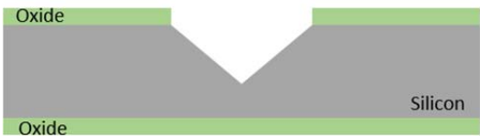
2) Silicon KOH etching to form V-groove
