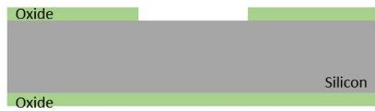
1) Oxide deposition and patterning
