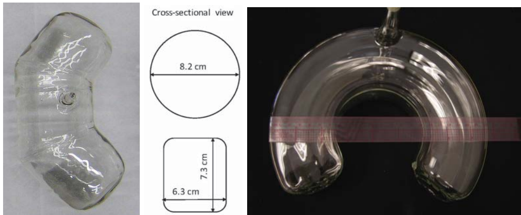
Figure 2. (Color online) Three-sectioned wide-angle cell as developed[11] (left photo). Each cell covers a scattering angle range between 90^\circ and 110^\circ ; An example of the recently developed horseshoe shaped wide angle cells (right photo). A cross-sectional view of both cells is shown in the middle of the photo. A circular cross section indicates the three-sectioned cell and a rectangular cross section indicates the horseshoe-shaped cell. A single horseshoe cell covers scattering angle of up to 260^\circ . The cell Mozart has an outside diameter of 23 cm, an inner diameter of 9.2 cm and a height of 7.5 cm.
