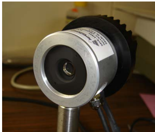
Fig. 6. Picture of a temperature controlled hybrid pyroelectric radiometer. The \text{LiTaO}_3 crystal is covered with organic-black coating.
