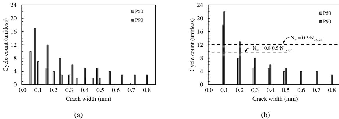
341 *Figure 3. Re-binning serviceability and suitability level protocols (example: cyclic crack width): (a) original cycle*
