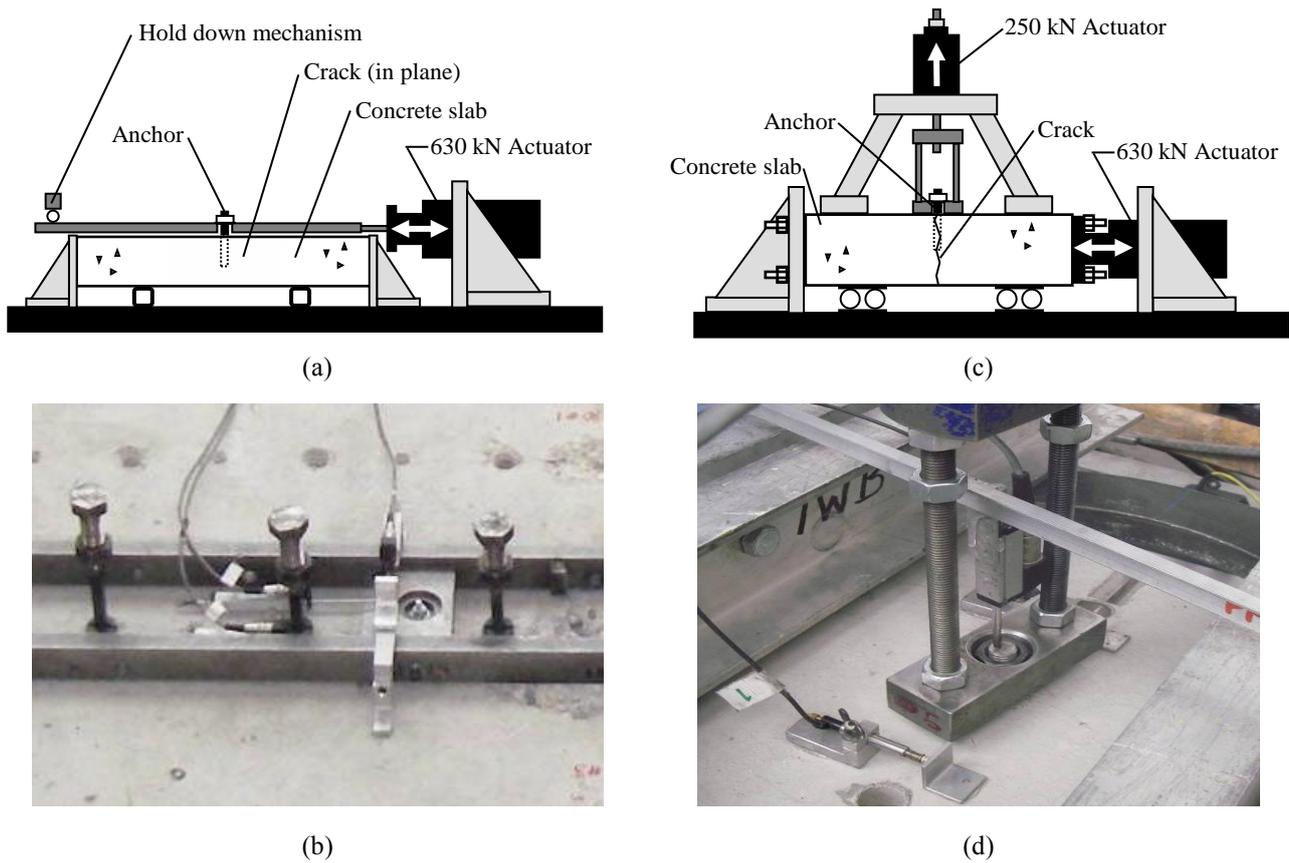
386 *Figure 5. Schematics and detailed views of the test setups: (a) and (b) cyclic shear; (c) and (d) cyclic crack tests.*
