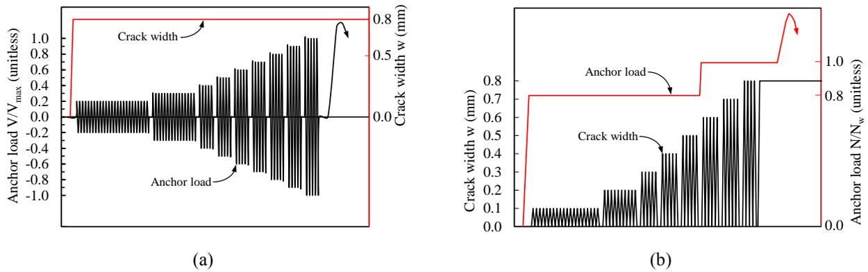
401 Figure 6. Unified test protocols: (a) cyclic shear load ( $V_{max} = 0.85 \cdot V_{u,cr,m}$ ); (b) cyclic crack ( $N_w = 0.5 \cdot N_{u,cr,m}$ ).
