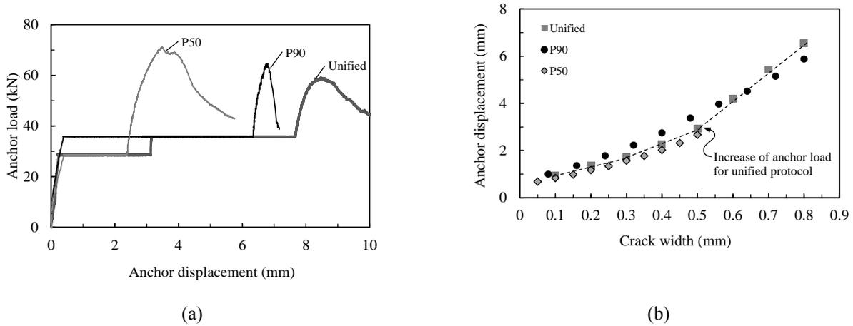
452 *Figure 8. Cyclic crack test on cast-in headed bolts: (a) example load displacement curve; (b) anchor*
