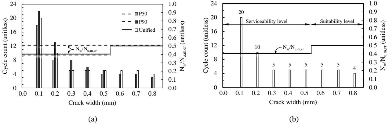
350 *Figure 4. Unifying serviceability and suitability level protocols (example: cyclic crack width): (a) relocated cycles for*
