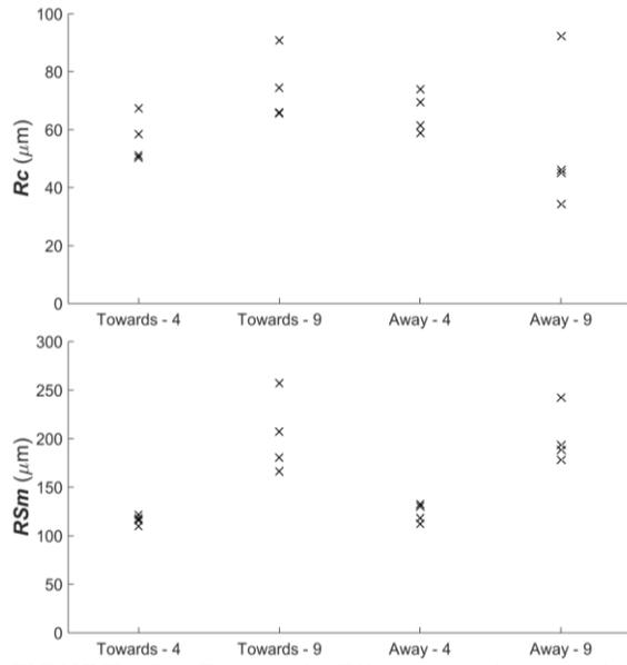
FIGURE 5.  $R_c$  and  $R_{Sm}$  for the vertical surfaces.
