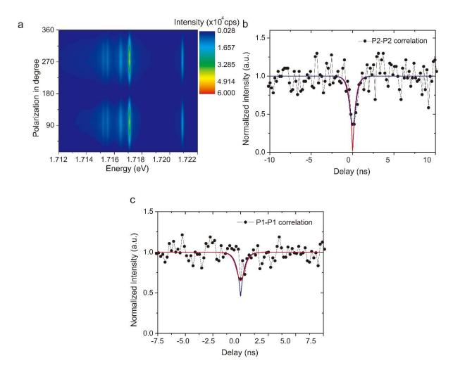
Supplementary Figure 5 | Polarization-resolved PL and photon antibunching.
