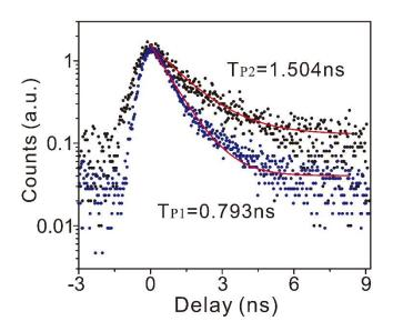
Supplementary Figure 4 Time-resolved Photoluminescence of P1 and P2 in one laser period (12.2ns). Compared to the XX, the X line is weak under higher excitation power and consequently it took longer time to perform the lifetime measurements. Thus the contribution of the APD (Avalanche Photon Diode) dark counts for the time resolved measurement on the X line is higher and results in an intensity offset.
