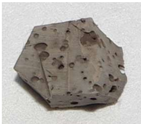
Figure S3. Backcoating residue after microscale combustion calorimetry. There is no surface manifestations of liquefaction (the sharp edges are incompatible with a liquefied material).
