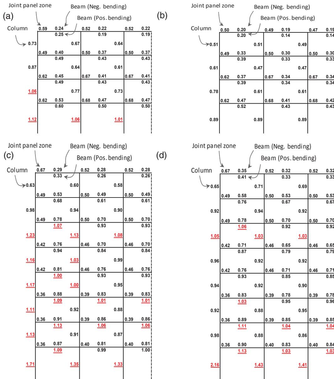
Fig. 4. Normalized demand-to-capacity ratio ( $DCR_N$ ) values for beams and columns in the interior E-W direction frame and beam-to-columns joints in the N-S direction frame at the Collapse Prevention performance level for: (a) 4-story ELF-designed building using LSP; (b) 4-story ELF-designed building using LDP; (c) 8-story ELF-designed building using LSP; (d) 8-story ELF-designed building using LDP. [Due to symmetry, the results are presented for half of the frame].
