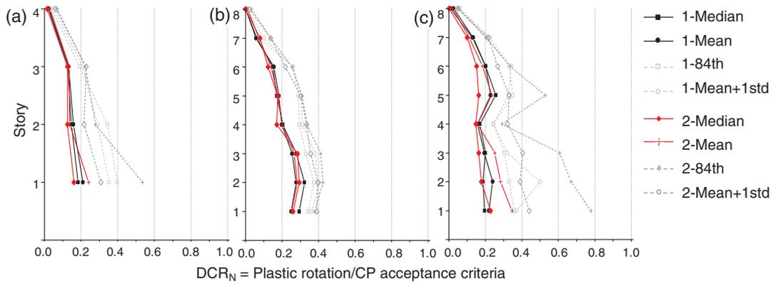
Fig. 9. Statistical information of the beam response assessed using NDP at the CP performance level for the (a) 4- story; (b) 8-story ELF-designed; (c) 8-story RSA-designed buildings. The results are presented for beams in the bay B-C of the E-W interior frame. [1- and 2-, in the legend, represent two ends of each beam.]
