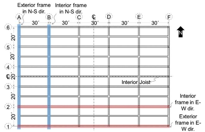
Fig. 1. (a) Plan view of the archetype building (1 ft = 0.3 m).
