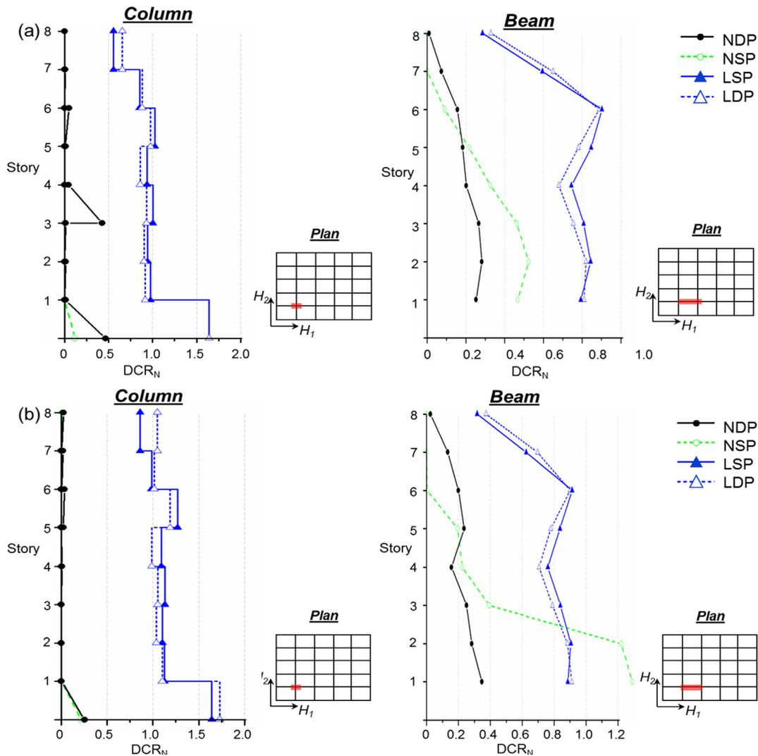
**Fig. 11.** Normalized demand-to-capacity ratio for selected beams and columns in the (a) 8-story ELF-designed and (b) 8-story RSA-designed frames using four evaluation procedures in Tier 3 analysis of ASCE 41. [For nonlinear procedures the average response is presented for columns; for beams the envelope of the response between two hinges at the end are shown.]
