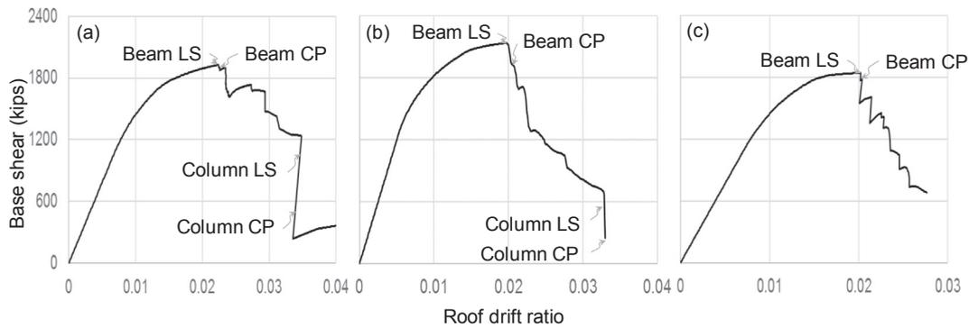
Fig. 6. Pushover analysis results in the E-W direction of the (a) 4-story; (b) 8-story ELF-designed; (c) 8-story RSA-designed frames (1 kip = 4.448 kN).
