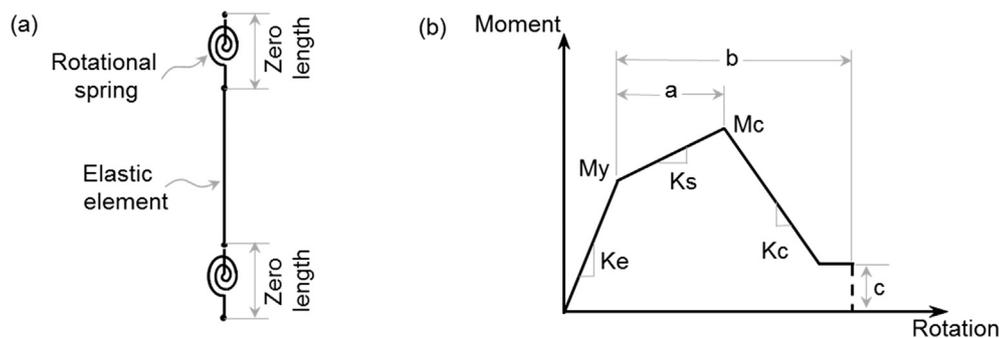
Fig. 2. Illustration of (a) column/beam flexural models implemented in P3D and (b) the column/beam flexural response.
