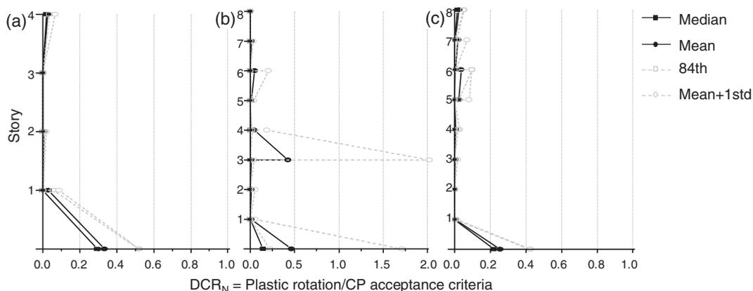
Fig. 10. Statistical information of the column response assessed using NDP at the CP performance level for the (a) 4- story; (b) 8-story ELF-designed; (c) 8-story RSA-designed buildings. The results are presented for columns at the intersection of intersection of grid lines 2 and C.
