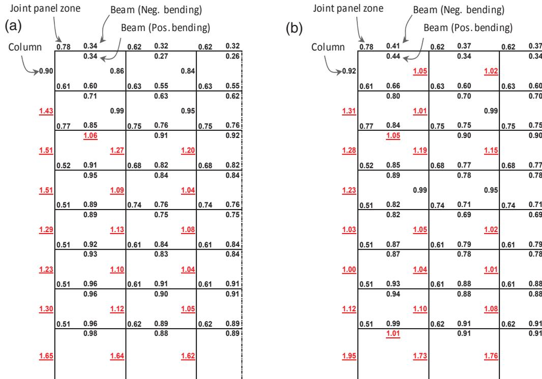
Fig. 5. Normalized demand-to-capacity ratio ( $DCR_N$ ) values for beams and columns in the interior E-W direction frame and beam-to-column joints in the N-S direction frame at the Collapse Prevention performance level for: (a) 8-story RSA-designed building using LSP, (b) 8-story RSA -designed building using LDP.
