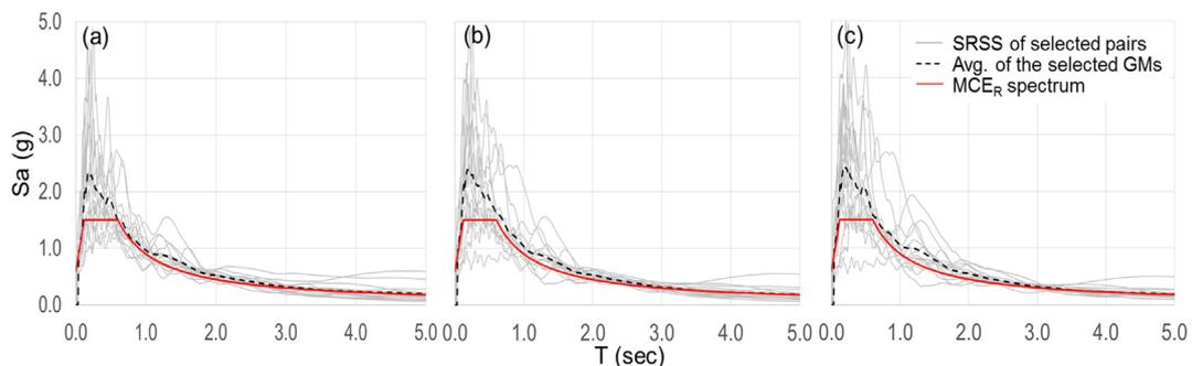
Fig. 8. Response spectra of selected scaled ground motions compared with the target spectrum for: (a) 4-story; (b) 8-story ELF-designed; (c) 8-story RSA-designed buildings.
