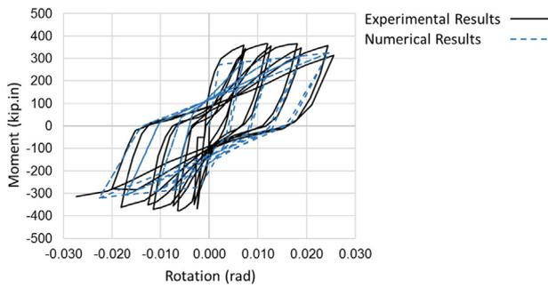
Fig. 3. Calibration of the cyclic response of the numerical model for a reinforced concrete beam (C5-00) tested by Matamoros [20] (1 kip = 4.448 kN, 1 in = 0.025 m).
