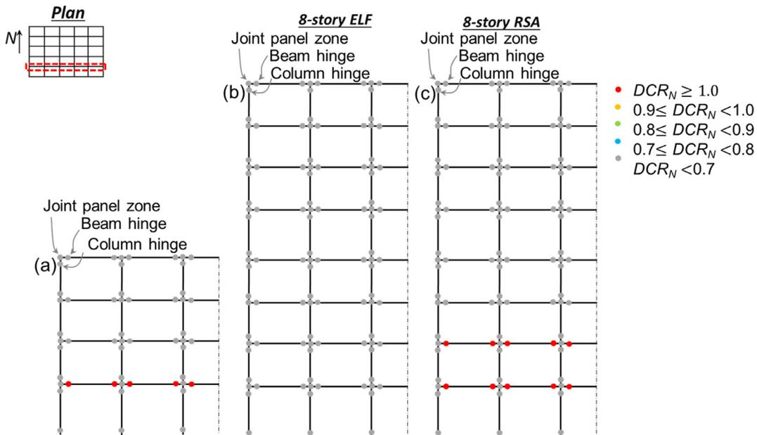
Fig. 7. Pushover analysis results for an interior frame in the E-W direction of the (a) 4-story; (b) 8-story ELF-designed; (b) 8-story RSA-designed frames.
