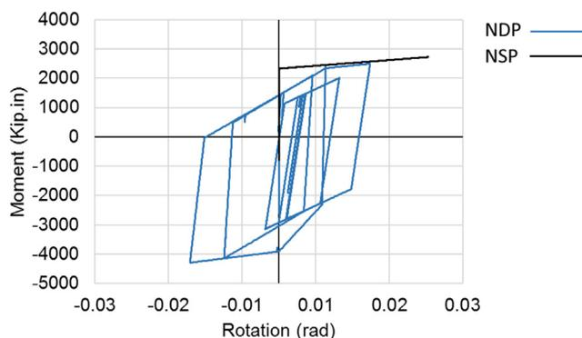
Fig. 12. Moment-rotation response of the left hinge of the beam shown in Fig. 11a for a single record in NDP (Imperial Valley EQ recorded at ElCentro) and the NSP results (1 kip = 4.448 kN, 1 in = 0.025 m). [The response for the NSP is terminated at the target displacement].
