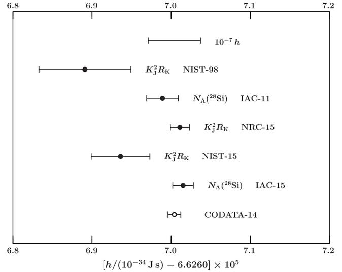
FIG. 4. Values of the Planck constant  $h$  with  $u_r < 10^{-7}$  inferred from the input data in Table XVIII and the 2014 CODATA recommended value in chronological order from top to bottom (see Table XXI). The input data from which these values are inferred are included in the final adjustment on which the 2014 recommended values are based.
