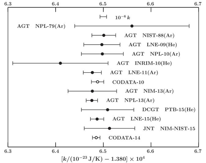
FIG. 5. Values of the Boltzmann constant  $k$  inferred from the input data in Table XVIII and the 2010 and 2014 CODATA recommended values in chronological order from top to bottom (see Table XXII). AGT: acoustic gas thermometry; DCGT: dielectric-constant gas thermometry; JNT: Johnson noise thermometry.
