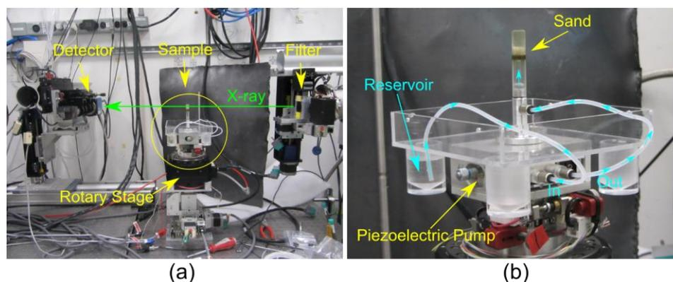
Figure 1: Experimental setup at APS 2-BM (a) and fluid flow experimental setup (b)
