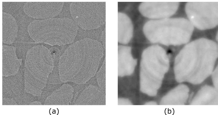
Figure 2: Reconstruction results using attenuation only (a) and phase retrieval (b)
