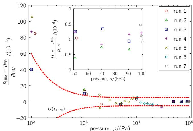
Fig. 2. Disagreement in pressure as measured by a laser refractometer ( $p_{\text{FP}}$ ) and ultrasonic manometer ( $p_{\text{UIM}}$ ); manometer uncertainty  $U(p_{\text{UIM}}) = [(6\text{ mPa})^2 + (5.2 \times 10^{-6} \cdot p)^2]^{1/2}$  also shown.
