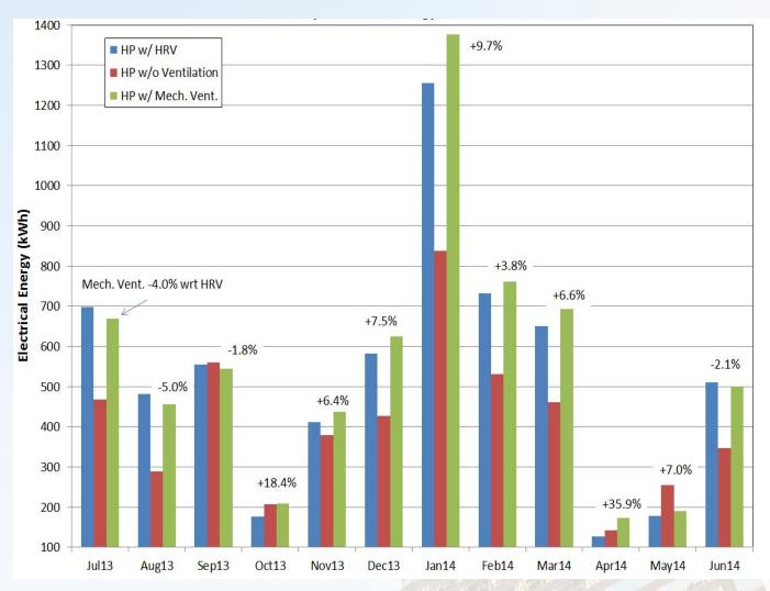
7 % savings in heat pump energy use on average over the year compared with ventilating without heat recovery
