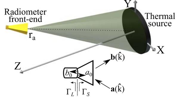
Fig. 1. Illustration of a radiometer collecting radiation from a blackbody and some notations for the plane-wave scattering matrix representing an antenna.
