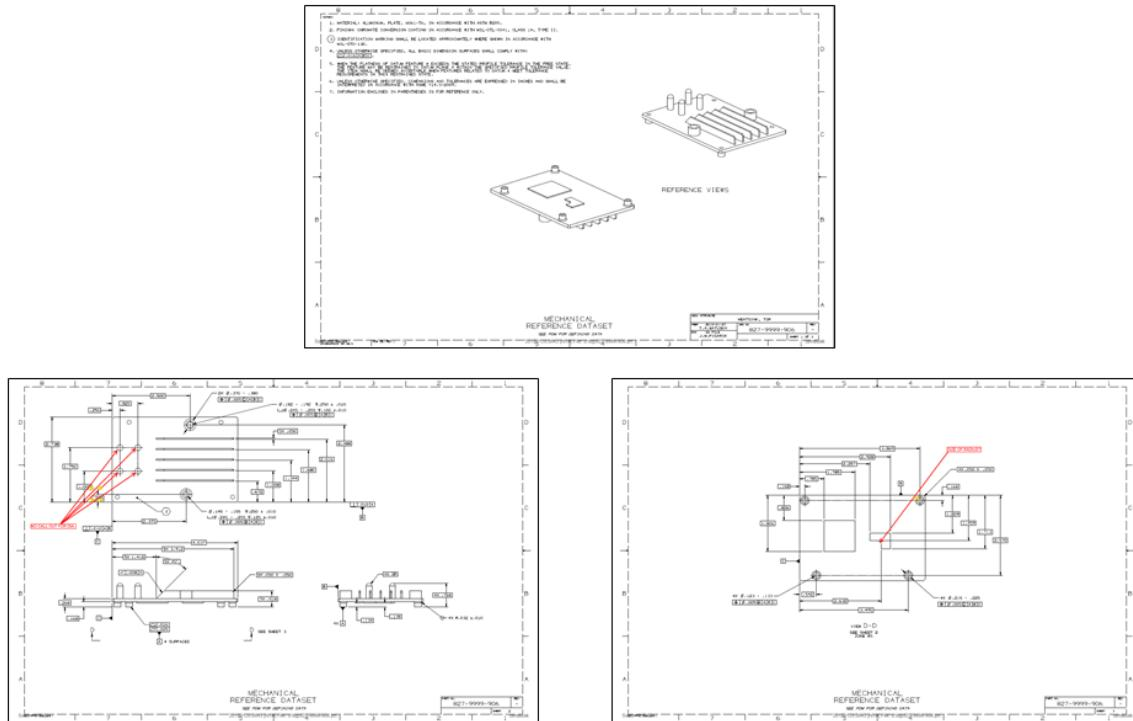
**Figure 12: CAD model creation - missing dimensions**
