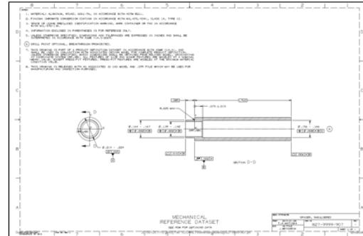
**Figure 5: Rolled Standoff 827-9999-907
