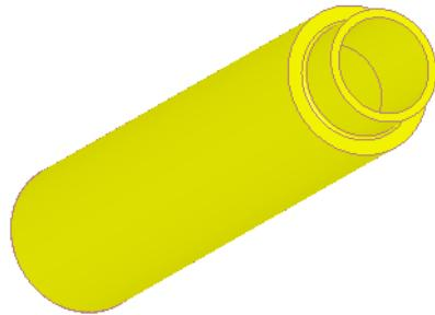
**Figure 1: Rolled Standoff**
