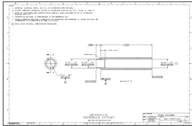
**Figure 3: Rolled Standoff 827-9999-905
