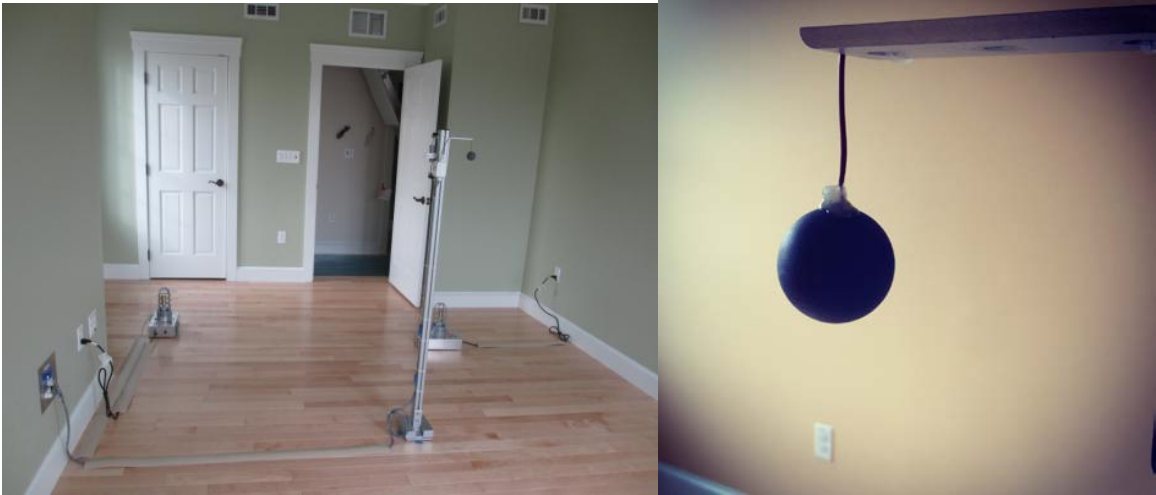
Figure 3. Thermal comfort sensors in room of the NZERTF (operative temperature probe on the right)
