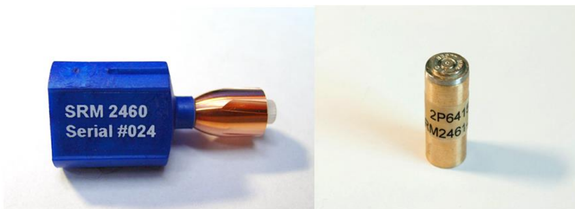
Figure 1: A SRM 2460 Standard Bullet (left) made by the numerically controlled (NC) diamond turning process and a SRM 2461 Standard Cartridge Case (right) made by the electro-forming technique. Both procedures are based on the techniques previously used for manufacturing surface roughness specimens.
