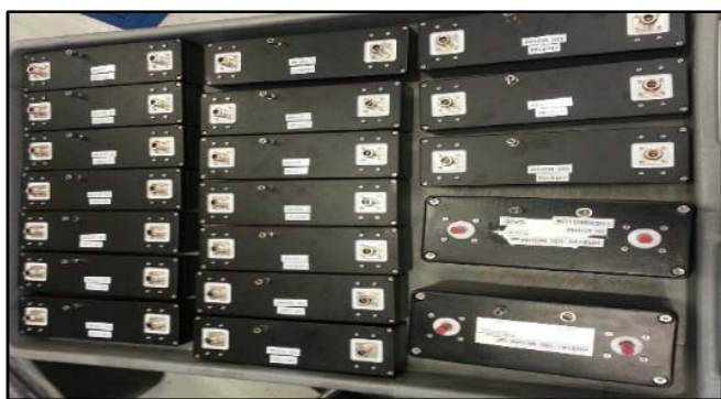
Fig. 2. Final Resistor assembly. 100 MΩ, 1 GΩ, 10 GΩ, and 100 GΩ resistors shown.
