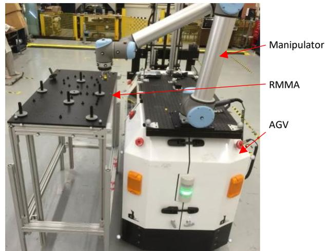
**Figure 3.** Docking performance measurement of a mobile manipulator with a reconfigurable mobile manipulator artifact (RMMA). Small spheres mounted on both the mobile manipulator and RMMA are used as fiducials for an optical ground truth system to measure mobile manipulator motion relative to the RMMA during test method development.
