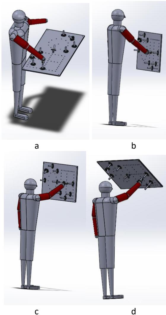
**Figure 6. Graphics of a human wearing arm exoskeletons (red) testing its performance using the RMMA for precision assembly applications when the RMMA is in (a) horizontal, (b) vertical-low, (c) vertical-high, and (d) overhead-angled configurations.**
