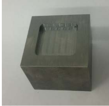
Figure 10. Part geometry for ordering different toolpath strategies
