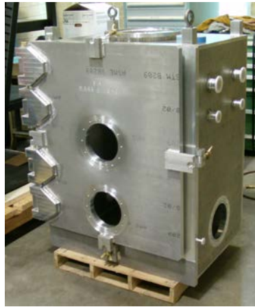
Figure 3: Upper Vacuum Chamber under construction.
