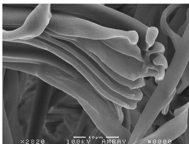
Figure 1. An SEM image of a Winged Fiber cross section.
