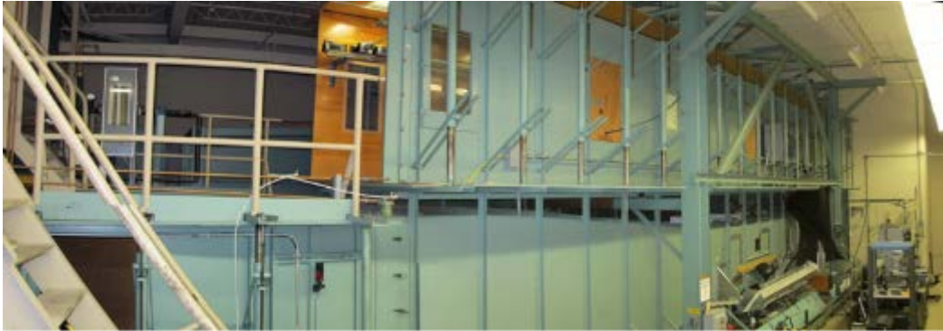
Figure 6 NIST wind tunnel used for calibration of S-type, L-type, and 3D pitot probes.
