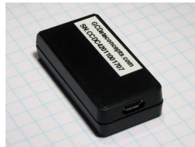
Fig. 2. X16-mini triaxial accelerometer
