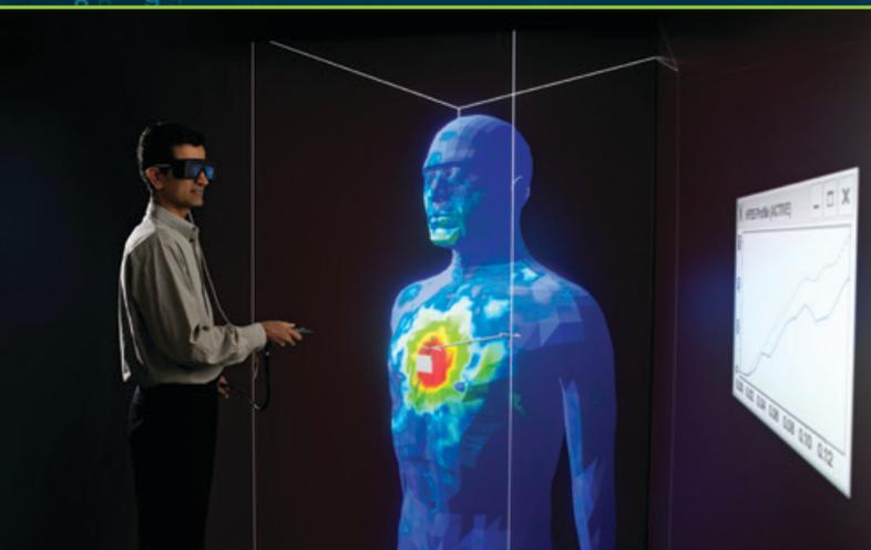
Computer engineer Kamran Sayrafian uses NIST's Reconfigurable 3D Immersive Platform to study and model how radio frequency (RF) waves propagate through the human body. This research supports the development of standards from implantable and wearable wireless medical devices.
