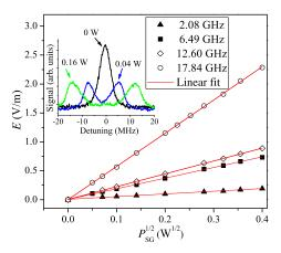
FIG. 3. Experimental data for rf E-field amplitude with a cubic vapor cell with 8-mm inner diameter as a function of the square root of power at the rf signal generator. The inset shows raw data for 2.08 GHz.
