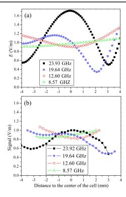
FIG. 7. rf E-field pattern in the cubic vapor cell with 8-mm inner diameter and 1-mm wall thickness. (a) The results of the 3D FE model for a 1 V m $^{-1}$  incident E-field. (b) The experimental results.
