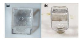
FIG. 2. The vapor cells used in the experiment. (a) The vapor cell with 8-mm inner diameter and 1-mm wall thickness. (b) The vapor cell with 9-mm inner diameter and 1.25-mm wall thickness.
