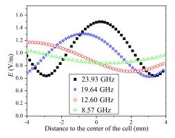
FIG. 6. One-dimensional model results for the E-field variability between two 1-mm-thick Pyrex walls separated by 8 mm for different frequencies for a 1 V m<sup>-1</sup> incident E-field.
