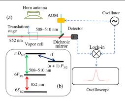
FIG. 1. Setup and energy-level diagram for the experiments. (a) The experimental setup. The probe and coupling lasers are overlapped inside the vapor cell and the rf horn antenna is placed in the far-field limit. (b) The energy-level diagram. The 852-nm and (508–510)-nm lasers are the EIT probe and coupling lasers, respectively. The rf E-field couples to the  $nD_{5/2} \leftrightarrow (n+1)P_{3/2}$  transitions.
