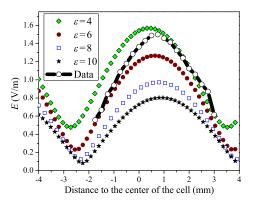
FIG. 5. One-dimensional model results for the E-field variability between two 1-mm-thick Pyrex walls separated by 8 mm for different dielectric constants at 23.93 GHz. The incident E-field is 1 V m<sup>-1</sup>.
