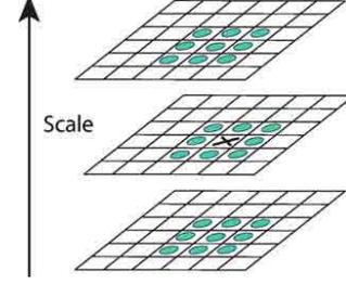
**Fig. 1:** Maxima and minima of the DoG images are detected by comparing a pixel( $X$ ) to its 26 neighbors in  $3 \times 3$  regions at the current and adjacent scales [5].
