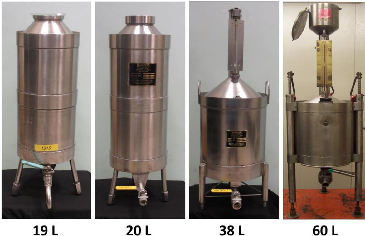
**Figure 3.** Four test measures used to measure retained volume dependence on kinematic viscosity.
