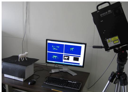
**Figure 1:** Setup for range scanning.
