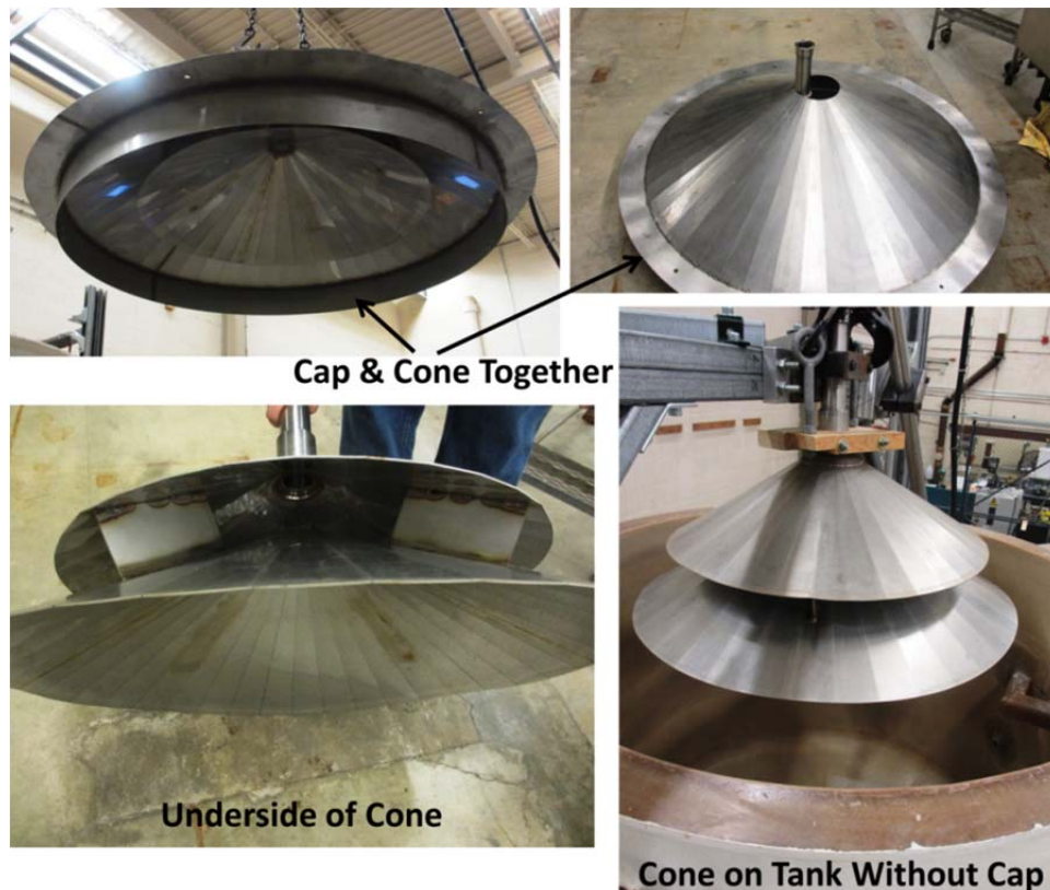
Fig. 4. The cover and cone removed from the collection tank. The cover rests on the collection tank without touching the cone that is used to direct the liquid into the tank. The incoming liquid flows between the two plates that make up the cone.
