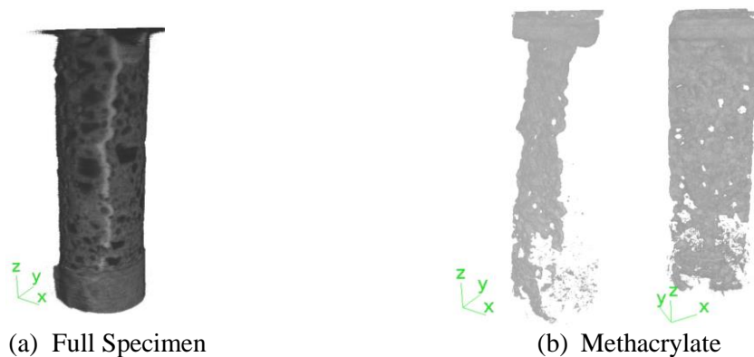
Figure 3: Neutron tomography of methacrylate filled crack. (a) extracted core and (b) mortar removed to show methacrylate (two views of the same crack).
