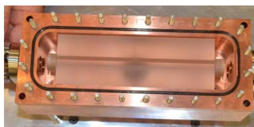
Fig. 5. The copper thermal shell/chamber (top lid removed) is built so there is a 1 mm gap between the ultralow expansion glass Fabry-Pérot cavity (center) and the chamber wall, and is designed to hold the temperature nearly constant while the cavity is filled with gas.
