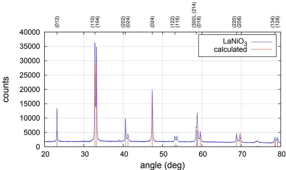
Figure 2: Diffractogram of the LaNiO<sub>3</sub> sample compared with peak positions and intensities computed from the known crystal structure.
