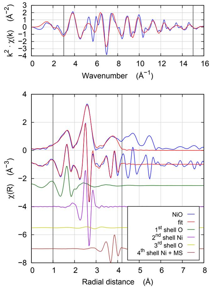
Figure 3: Fit to NiO using the cubic halite structure. The brown line includes the contribution from the fourth shell Ni scatterer plus several collinear MS paths at the same distance. The vertical lines show the ranges of the Fourier transform in  $k$  and the fit in  $R$ .
