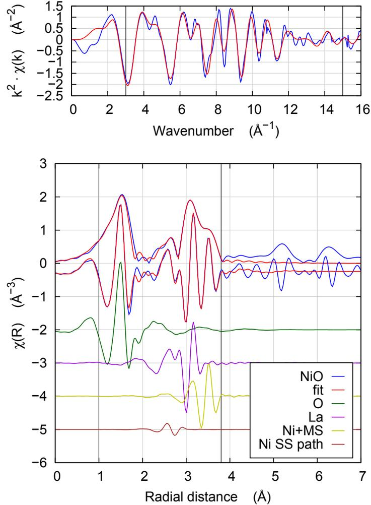
Figure 4: Fit to LaNiO<sub>3</sub> using the constructed Ni SS path. The yellow line includes contributions from the third shell Ni scatterer plus several multiple scattering paths at the same path length. The brown line is the Ni SS path added to represent the contribution from the non-diffracting Ni oxide. The vertical lines show the ranges of the Fourier transform in  $k$  and the fit in  $R$ .
