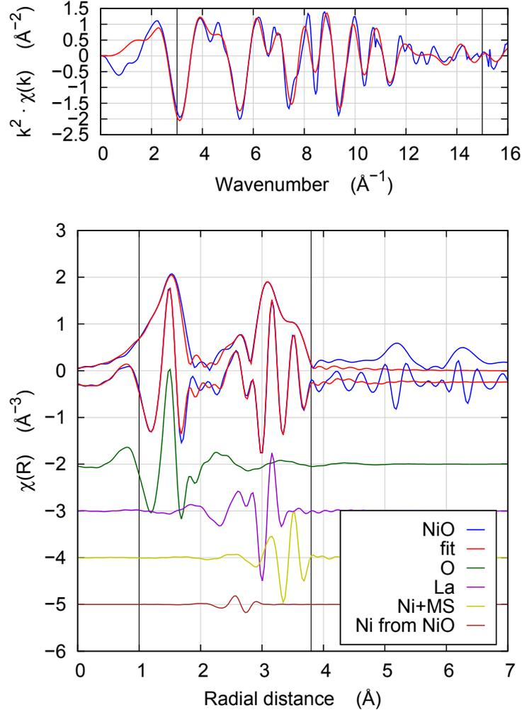
Figure 5: Fit to LaNiO<sub>3</sub> using the 2<sup>nd</sup> shell Ni path from NiO. The yellow line includes contributions from the third shell Ni scatterer plus several multiple scattering paths at the same path length. The brown line is the 2<sup>nd</sup> shell Ni path from NiO used to account for the non-diffracting Ni oxide. The vertical lines show the ranges of the Fourier transform in  $k$  and the fit in  $R$ .
