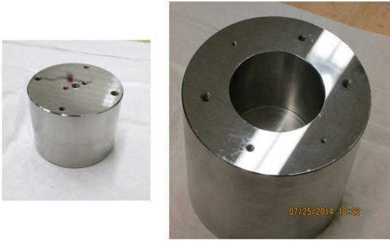
Fig. 3. Specific load mass objects for which elastic properties were measured and more-detailed simulations carried out. The object on the left has a mass of approximately 1 kg, a diameter of \approx 0.06 m, and a height of \approx 0.045 m. The object on the right has a mass of approximately 10 kg, a diameter of \approx 0.12 m, a height of \approx 0.13 m and an internal cavity of depth \approx 0.06 m. In addition to the holes shown, each mass had a threaded hole in its base of diameter 6.4 mm and depth \approx 20 mm.
