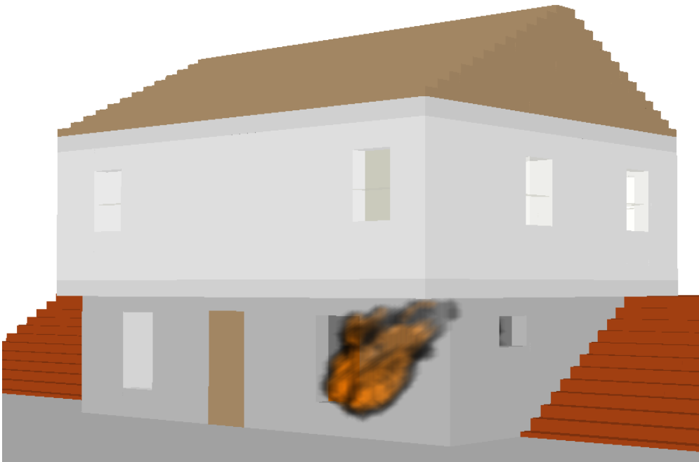
Figure 4.3: External post-fire image of damage to the basement (top) and FDS model showing external fire prior to the front door of the structure being opened (bottom).
