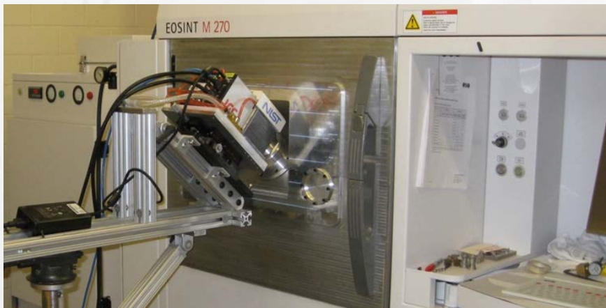
Thermal camera looking into the viewport
