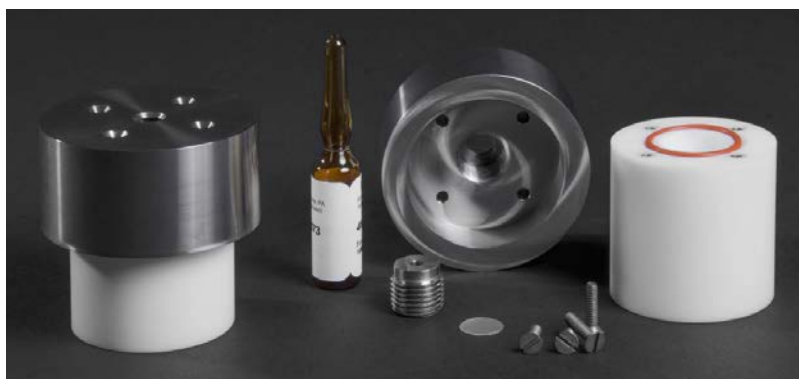
Figure 1: NIST formaldehyde reference standard (FRS). The FRS consists of a formalin ampule, a stainless steel lid, a compression set screw, a polydimethylsiloxane (PDMS) membrane, four stainless steel screws, a Teflon base with 3 mL formalin well, and an O-ring. The lid is sealed to the bottle with the screws.
