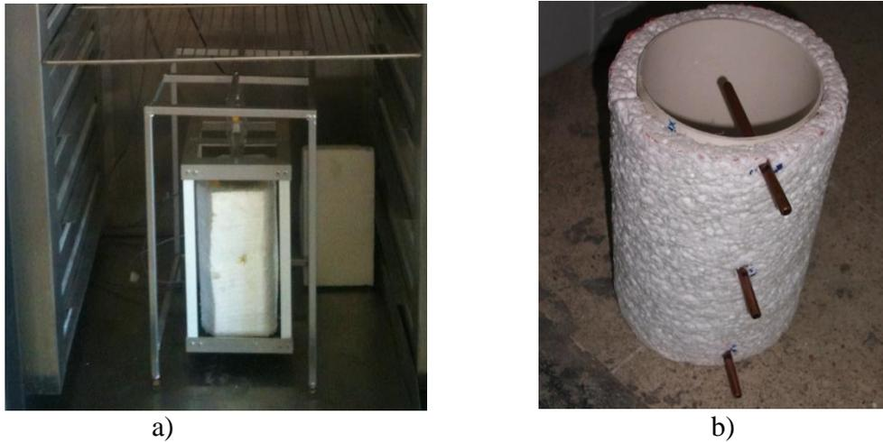
Figure 4. a) Experimental setup inside the environmental chamber, and b) Polystyrene insulated PVC mold for Type B specimens, showing only three of the seven holes for the thermocouples.
