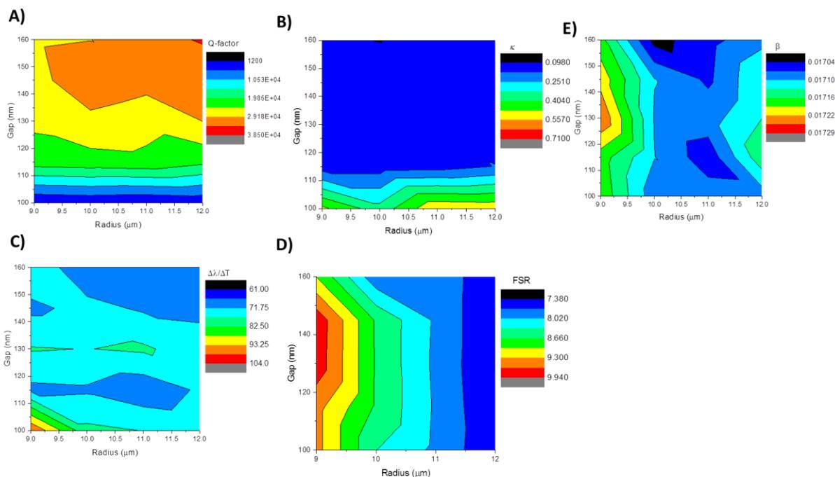
**Fig. 1:** Impact of structural parameters on a) FSR b) Q-factors c) temperature response d) propagation constant and e) coupling loss.
