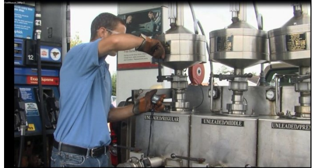
Figure 6 – Inspector Draining a Prover
