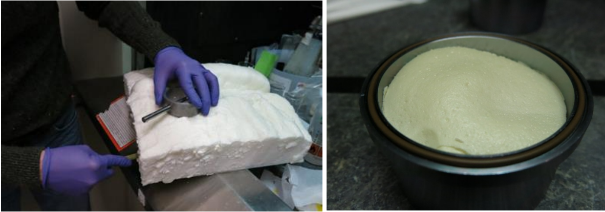
Figure 1. Sampling of foam Open 1 for micro-chamber analysis (left). Sample installed in micro chamber (right).
