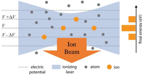
Figure 3 Schematic view showing the origin of the chromatic energy spread in LoTIS. Ions are created over a finite extent in a non-zero electric field. The differences in the potentials at which they are created give rise to the chromatic energy spread.
