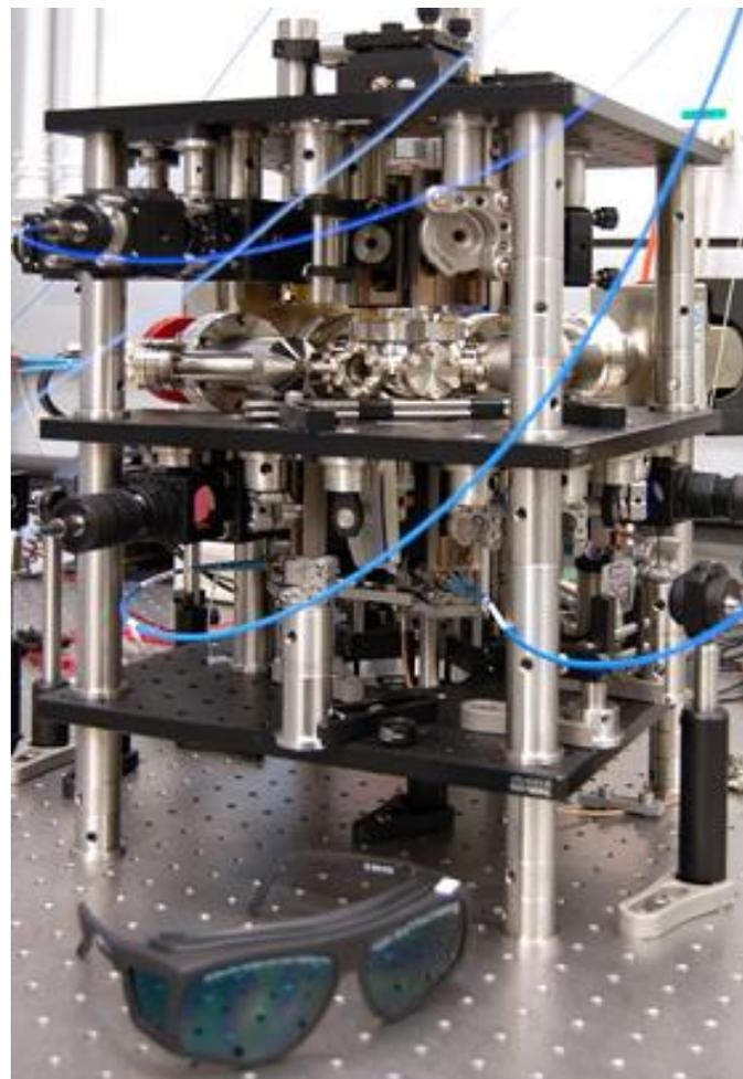
Figure 2: Photograph of Low Temperature Ion Source (LoTIS) prototype. Laser safety glasses included in foreground for scale. Lasers used to power the source are located on another table and light is carried to the source through fiber optics. The prototype shown includes all the components needed to create the ion source, but does not include an ion focusing column or a sample chamber
