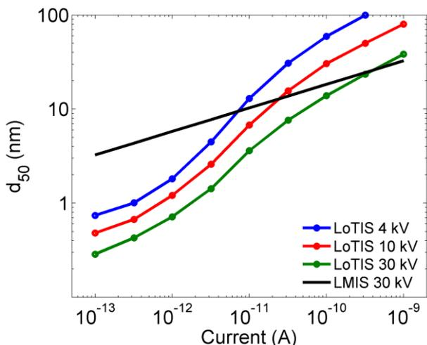
Figure 5 Projected performance of the LoTIS for beam energies of 4 kV, 10 kV and 30 kV, and LMIS data at 30 kV.  $d_{50}$  is the diameter into which 50% of the total beam current falls in the focal plane. The plot shows currents between 0.1 pA and 1 nA.
