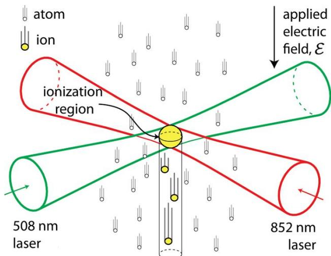
Figure 1 Ionization laser geometry, showing the overlapping 852 nm 508 nm lasers driving the two-step photoionization.
