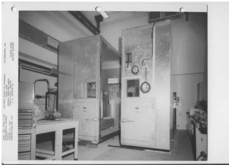
Figure 7 NBS hot box test apparatus 1967 - 1980
