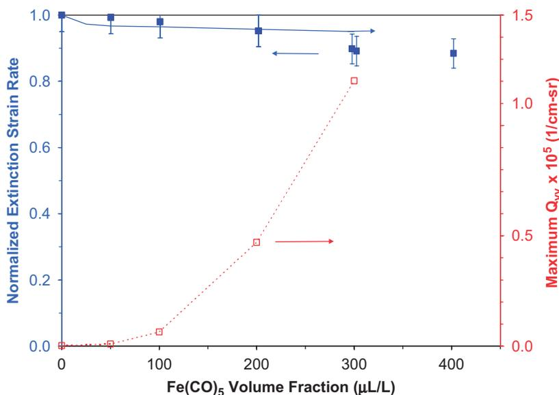
Fig. 31. Effect of  $\text{Fe}(\text{CO})_5$  added to the fuel stream of a methane-air counterflow diffusion flame. The experimentally measured and numerically calculated normalized extinction strain rate [43] are shown (left axis) as a function of  $\text{Fe}(\text{CO})_5$  volume fraction in the fuel stream. The maximum scattering cross section (right axis), obtained from the results in Fig. 30 is also shown for increasing  $X_{\text{inh}}$ .
