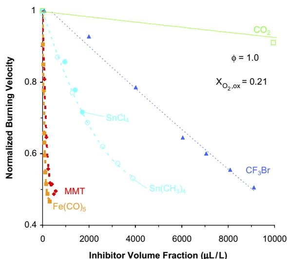
Fig. 16. Normalized burning velocity of premixed  $\text{CH}_4/\text{O}_2/\text{N}_2$  flames inhibited by  $\text{CO}_2$ ,  $\text{CF}_3\text{Br}$ ,  $\text{Sn}(\text{CH}_3)_4$ ,  $\text{SnCl}_4$  [49], MMT, and  $\text{Fe}(\text{CO})_5$  ( $T_{\text{in}} = 353 \text{ K}$  for all data except  $\text{Sn}(\text{CH}_3)_4$  and  $\text{SnCl}_4$  which are at  $298 \text{ K}$ ) (points: experiments; lines: curve fits) [10].
