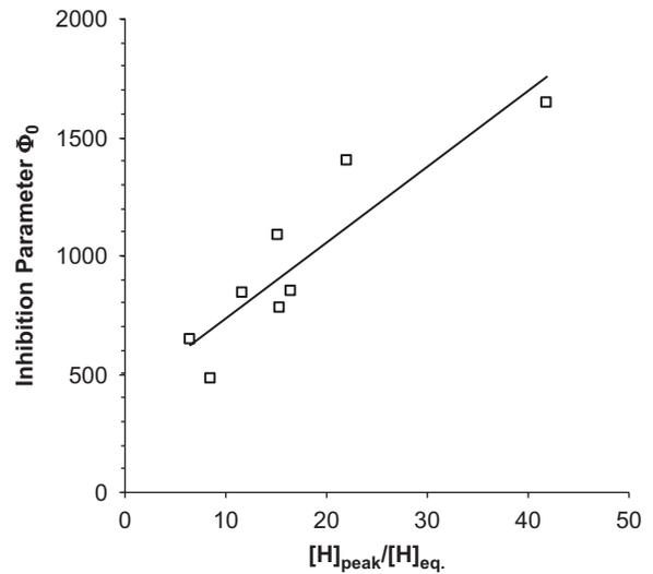
Fig. 5. Variation of inhibition parameter  $\Phi_0$  [124] with degree of H-atom super equilibrium in premixed methane–air flames with added Fe(CO)<sub>5</sub> (line: linear curve fit) [9].
