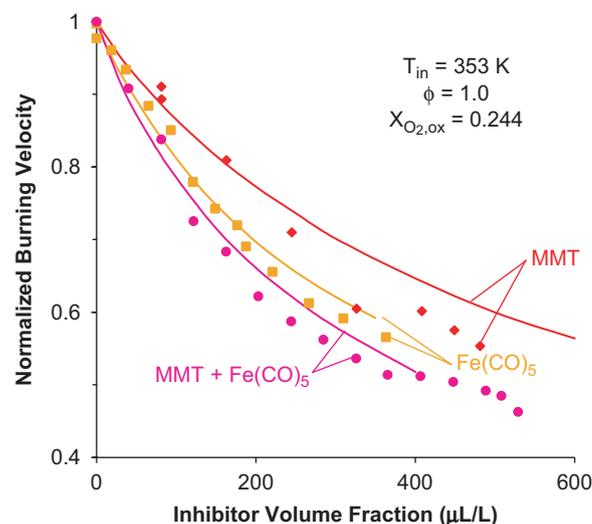
Fig. 21. Normalized burning velocity of premixed  $\text{CH}_4/\text{O}_2/\text{N}_2$  flames inhibited by pure MMT and  $\text{Fe}(\text{CO})_5$ , and by a blend of the two (points: experiments; lines: numerical calculations) [10].
