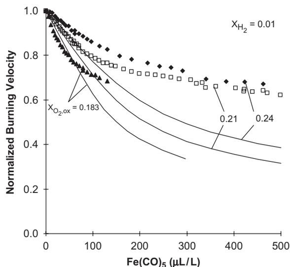
Fig. 9. Normalized burning velocity for CO/O<sub>2</sub>/H<sub>2</sub>/N<sub>2</sub> flames with added Fe(CO)<sub>5</sub> with  $X_{H_2} = 0.01$  and varying  $X_{O_2,ox}$  (points: experiments; lines: numerical calculations) [74].
