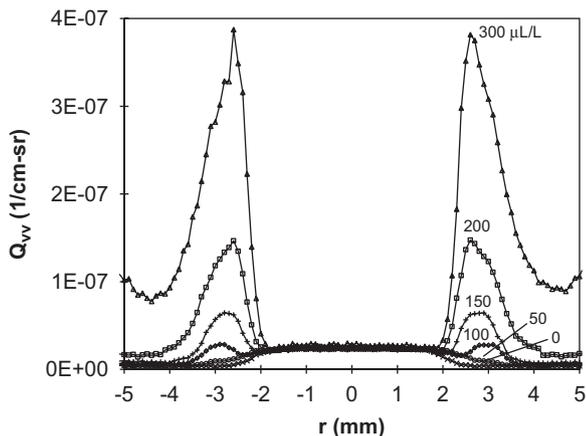
Fig. 23. Measured scattering cross section through a stoichiometric  $\text{CH}_4$ -air flame 7 mm above the burner rim at various inhibitor volume fractions [41].
