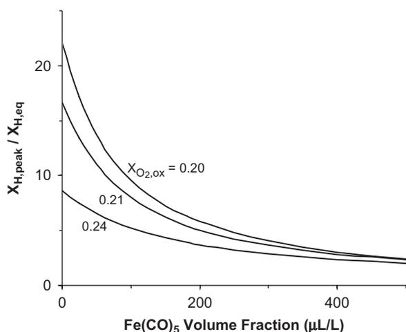
Fig. 14. Calculated ratio of peak and equilibrium values of  $[\text{H}]$  in premixed  $\text{CH}_4/\text{O}_2/\text{N}_2$  flames with added  $\text{Fe}(\text{CO})_5$  at different  $X_{\text{O}_2,\text{ox}}$  [42].
