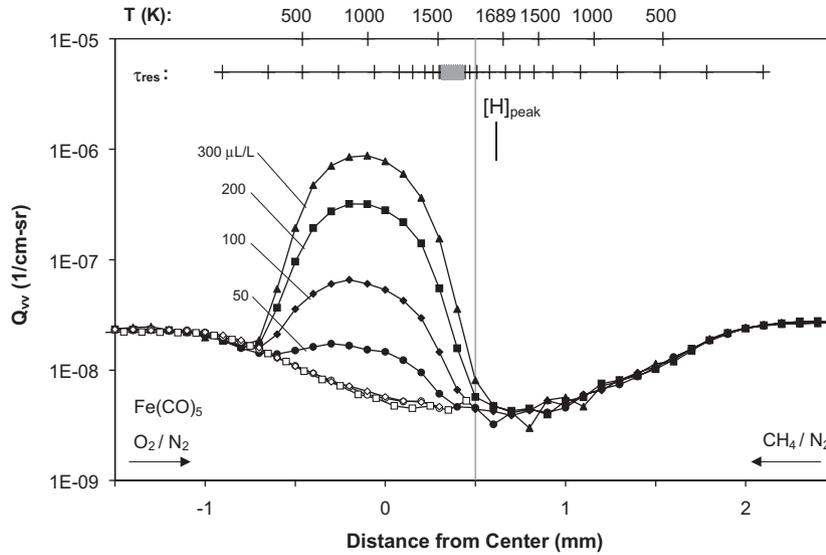
Fig. 32. Scattering profiles through a counterflow diffusion flame of 30%  $O_2/70\%$   $N_2$  and 80%  $CH_4/N_2$ . The calculated temperature and point of peak H-atom mole fraction are marked on the upper  $x$ -axis, and the vertical line denotes the calculated location of the stagnation plane.  $Fe(CO)_5$  is added to the oxidizer stream at the indicate volume fraction. The estimated residence time for 5 nm particles is shown as 10 ms intervals in the hatched line near the top [45].
