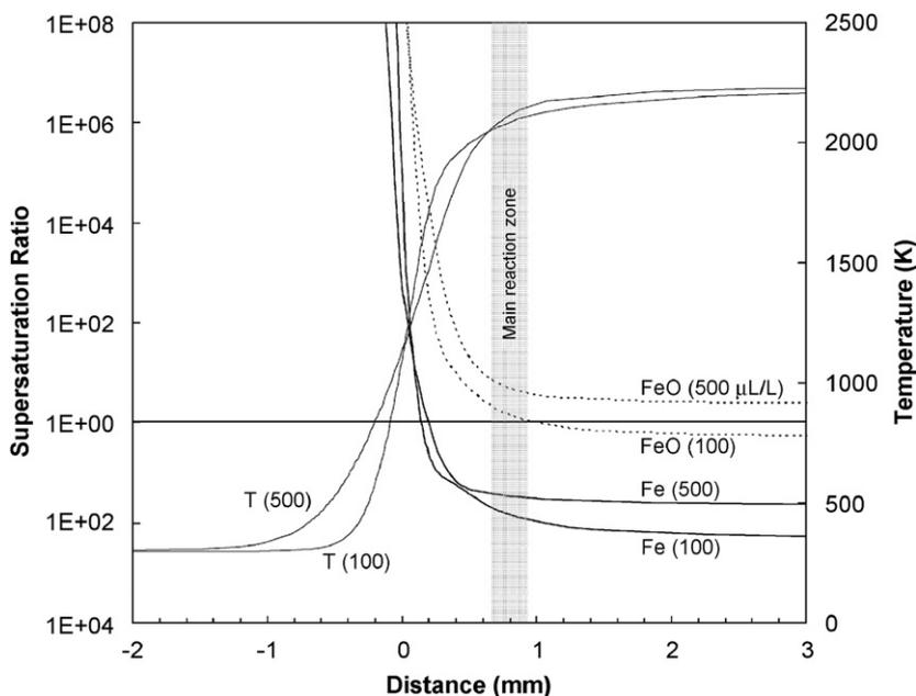
Fig. 15. Temperature and supersaturation ratio of Fe and FeO as a function of position through a premixed  $\text{CH}_4$ -air flame with  $\text{Fe}(\text{CO})_5$  added at 100 or 500  $\mu\text{L}/\text{L}$  [9].
