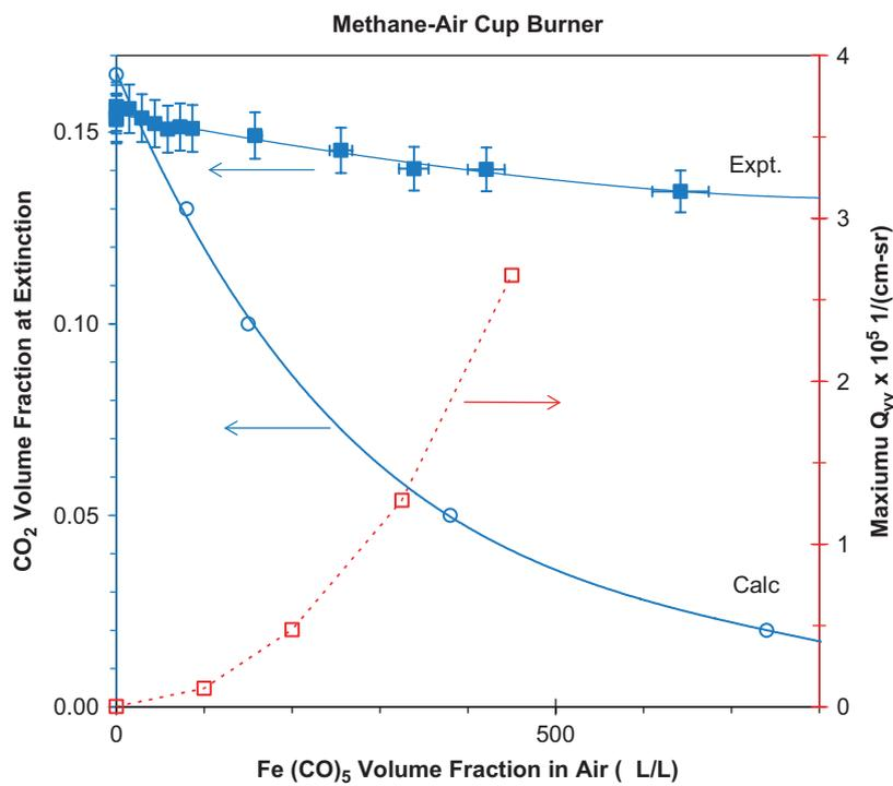
Fig. 38. Experimental and numerically predicted extinction volume fraction of CO<sub>2</sub> (left axis) and peak measured scattering cross section (right axis), as a function of the volume fraction of Fe(CO)<sub>5</sub> in the air stream [115,138].
