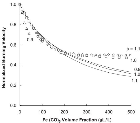
Fig. 4. Normalized burning velocity of premixed CH<sub>4</sub>–air flames with added Fe(CO)<sub>5</sub> at varying φ (points: experimental data; lines: 1-D numerical predictions with gas-phase inhibition chemistry) [9].
