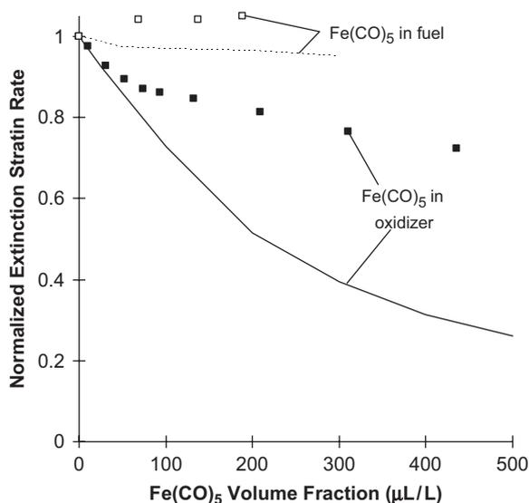
Fig. 7. Normalized extinction strain rate for  $\text{CH}_4/\text{O}_2/\text{N}_2$  flames with added  $\text{Fe}(\text{CO})_5$  in the oxidizer stream or fuel stream (points: experiment; lines: numerical calculation) [9].
