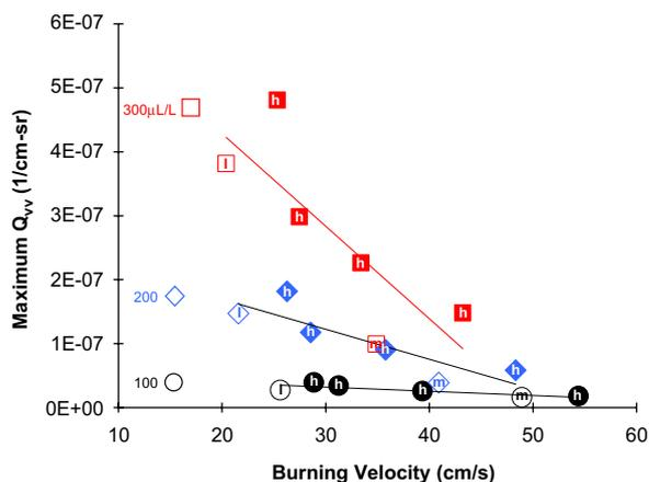
Fig. 26. Maximum  $Q_{vv}$  for flames of CH<sub>4</sub> (open symbols) and CO (closed symbols) as a function of the burning velocity. The letters correspond to the adiabatic flame temperature (low, medium, and high: 2220, 2350, and 2470 K), while the symbol shape (square, diamond, and circle) corresponds to the loading of Fe(CO)<sub>5</sub>: (100, 200, and 300) μL/L [41].
