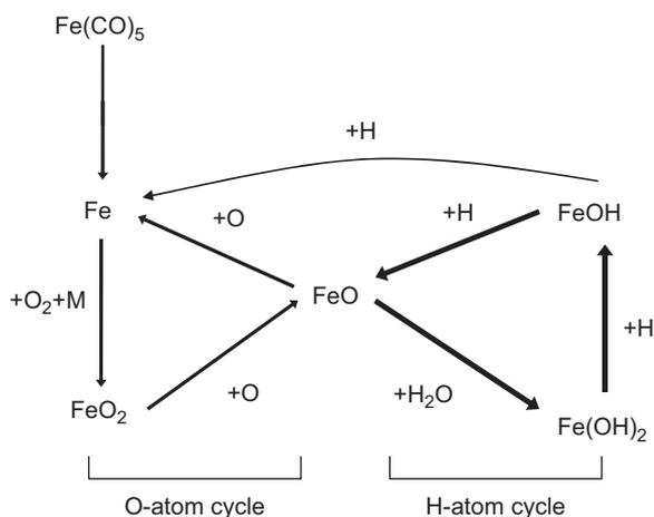
Fig. 12. Schematic diagram of radical recombination reaction pathways is found to be important for  $\text{CO}/\text{H}_2/\text{O}_2/\text{N}_2$  flames. Thicker arrows correspond to higher reaction flux. Reaction partners are listed next to each arrow [74].
