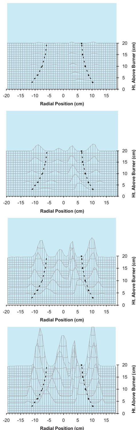
Fig. 35. Scattering cross section for laser light at 488 nm as a function of radial position and height above burner in methane–air cup-burner flame with 8%  $\text{CO}_2$  and  $\text{Fe}(\text{CO})_5$  in air at specified volume fraction. Dotted lines show flame location from a digitized video image of the uninhibited flame [115]. Top to bottom frames have (100, 200, 325, and 450)  $\mu\text{L}/\text{L}$  of  $\text{Fe}(\text{CO})_5$ , respectively.
