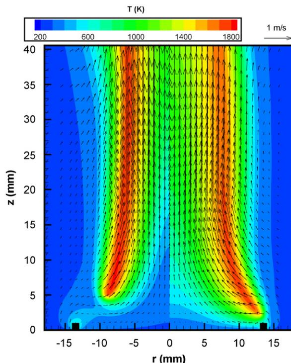
Fig. 36. Calculated temperature (color scale) and velocity vectors (arrows) for methane–air cup-burner flame with an oxidizer stream  $\text{CO}_2$  volume fraction of 10%, with (left) and without (right) an added  $\text{Fe}(\text{CO})_5$  volume fraction of 100  $\mu\text{L}/\text{L}$  [115].
