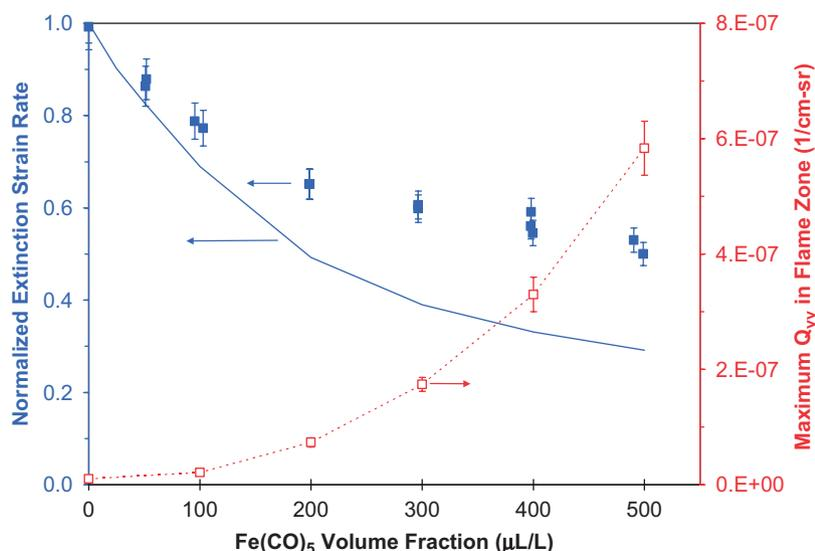
Fig. 29. Correlation between inhibition effect and maximum  $Q_{vv}$ . Filled points are experimental normalized  $a_{\text{ext}}$ , solid line is calculated  $a_{\text{ext}}$  [43]. Open symbols connected by dotted lines are maximum measured  $Q_{vv}$ . Particle data collected at 75% of  $a_{\text{ext}}$  [45].
