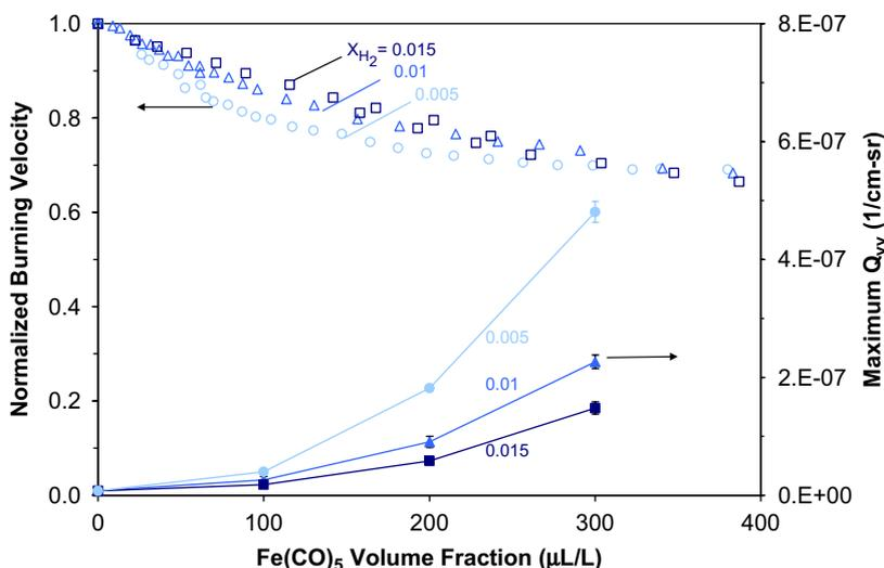
Fig. 25. Maximum scattering signal and normalized burning velocity [74] for CO–H<sub>2</sub> flames as Fe(CO)<sub>5</sub> concentration varies [41].
