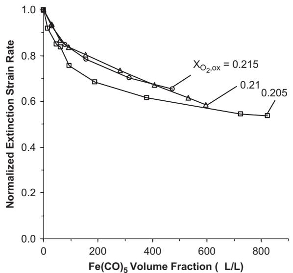
Fig. 6. Normalized extinction strain rate for CH<sub>4</sub>/O<sub>2</sub>/N<sub>2</sub> flames with added Fe(CO)<sub>5</sub> in the oxidizer stream having X<sub>O<sub>2,ox</sub></sub> = 0.205, 0.21, and 0.215 (lines and points: experiments) [9].
