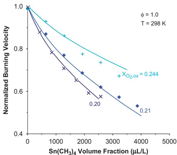
Fig. 17. Normalized burning velocity of premixed  $\text{CH}_4/\text{O}_2/\text{N}_2$  flames inhibited by TMT, with  $\phi = 1.0$  and  $X_{\text{O}_2,\text{ox}} = 0.20, 0.21,$  and  $0.244$  (points: experiments; lines: numerical calculations) [10].
