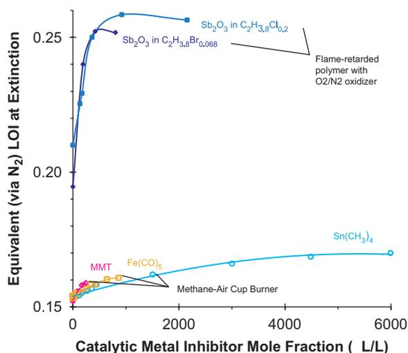
Fig. 41. Equivalent  $\text{N}_2/\text{O}_2$  limiting oxygen index for extinction of polyethylene (PE) halogen blends or methane–air cup burner flames with MMT,  $\text{Fe}(\text{CO})_5$ , and  $\text{Sn}(\text{CH}_3)_4$  [152].
