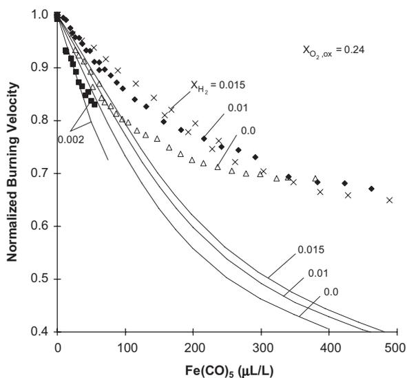
Fig. 10. Normalized burning velocity for CO/O<sub>2</sub>/H<sub>2</sub>/N<sub>2</sub> flames with added Fe(CO)<sub>5</sub> with  $X_{O_2,ox} = 0.24$  and varying  $X_{H_2}$  (points: experiments; lines: numerical calculations) [74].
