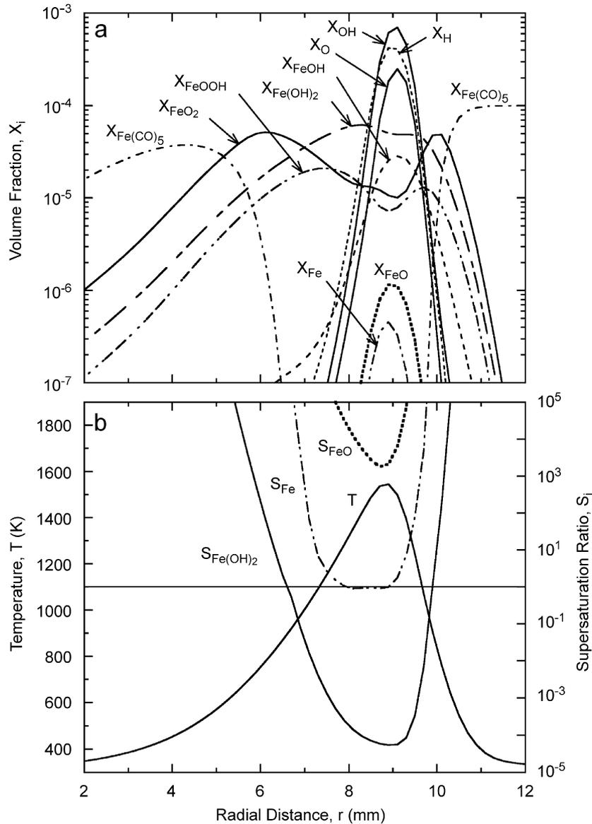
Fig. 39. (a) Calculated volume fraction  $X_i$  for iron-containing and major species as a function of radial position at the height above the burner of 4.8 mm (corresponding to the location of the reaction kernel in the flame base) and (b) the super-saturation ratio,  $S_i$ , for Fe, FeO, and Fe(OH)<sub>2</sub> [115].
