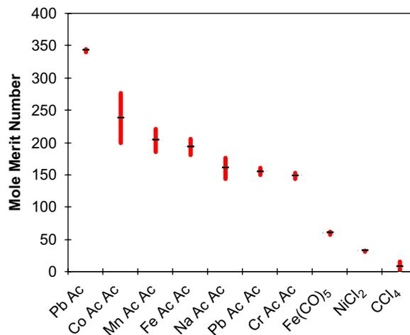
Fig. 1. Mole merit number of metal compounds for the oxidizer velocities in the range of 50–60 cm/s (from [73]).
