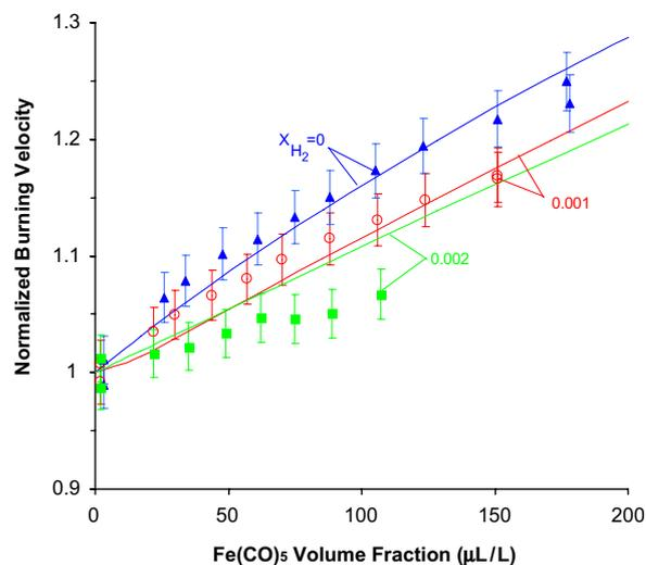
Fig. 11. Normalized burning velocity of premixed CO/N<sub>2</sub>O flames with varying hydrogen content, as a function of Fe(CO)<sub>5</sub> volume fraction (points: experiments; lines: numerical calculations) [103].
