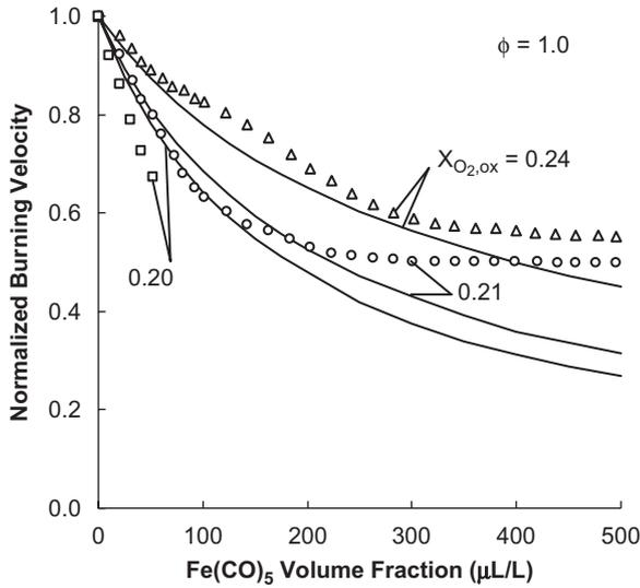
Fig. 3. Normalized burning velocity of premixed CH<sub>4</sub>–air flames with added Fe(CO)<sub>5</sub> at varying X<sub>O<sub>2,ox</sub></sub> (points: experimental data; lines: 1-D numerical predictions with gas-phase inhibition chemistry) [9].
