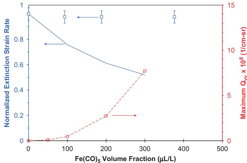
Fig. 33. Effect of  $Fe(CO)_5$  added to the air stream of a diluted methane–air counterflow diffusion flame. The experimentally measured (points) and numerically calculated (solid line) normalized extinction strain rate [43] are shown (left axis) as a function of  $Fe(CO)_5$  volume fraction in the air stream. The maximum scattering cross section (right axis), obtained from the results in Fig. 30 is also shown for increasing  $X_{inh}$  [50].
