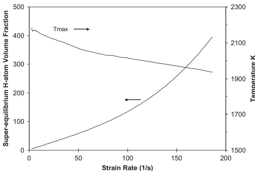
Fig. 8. Super-equilibrium ratio and temperature variation with strain for counterflow  $\text{CH}_4$ –air flames [151].
