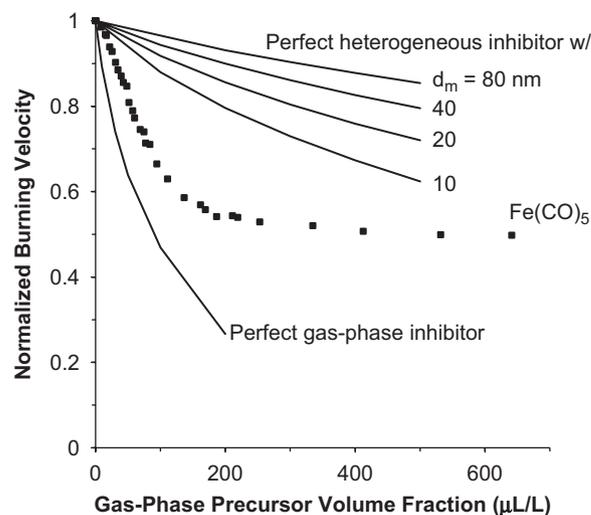
Fig. 27. Calculated normalized burning velocity for several diameters  $d_m$  of ideal heterogeneous inhibitor. Also shown are  $\text{Fe}(\text{CO})_5$  data and calculated normalized burning velocity using the perfect gas-phase inhibitor mechanism [41].
