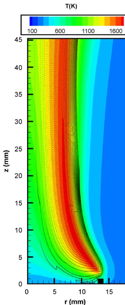
Fig. 40. Calculated particle trajectories for free-molecular-regime particles in a  $\text{CH}_4$ -air flame with 10%  $\text{CO}_2$  in the oxidizer stream [115].
