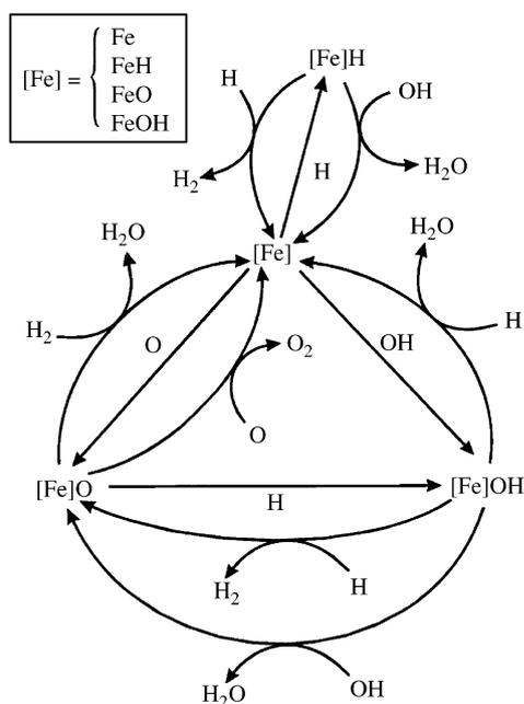
Fig. 13. Schematic representation of different classes of reactions which may contribute to iron's super-efficient flame suppression ability through the catalytic recombination of radical species [111].
