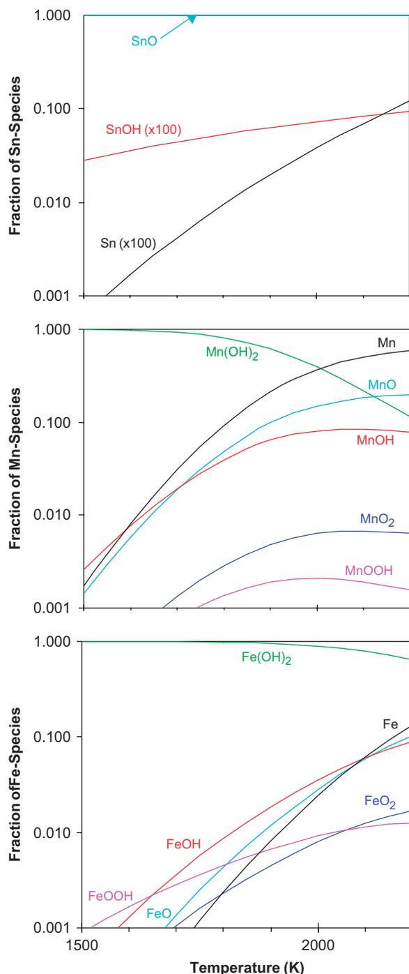
Fig. 20. Fraction of Sn-, Mn-, and Fe-species at equilibrium in methane-air flames as a function of temperature.
