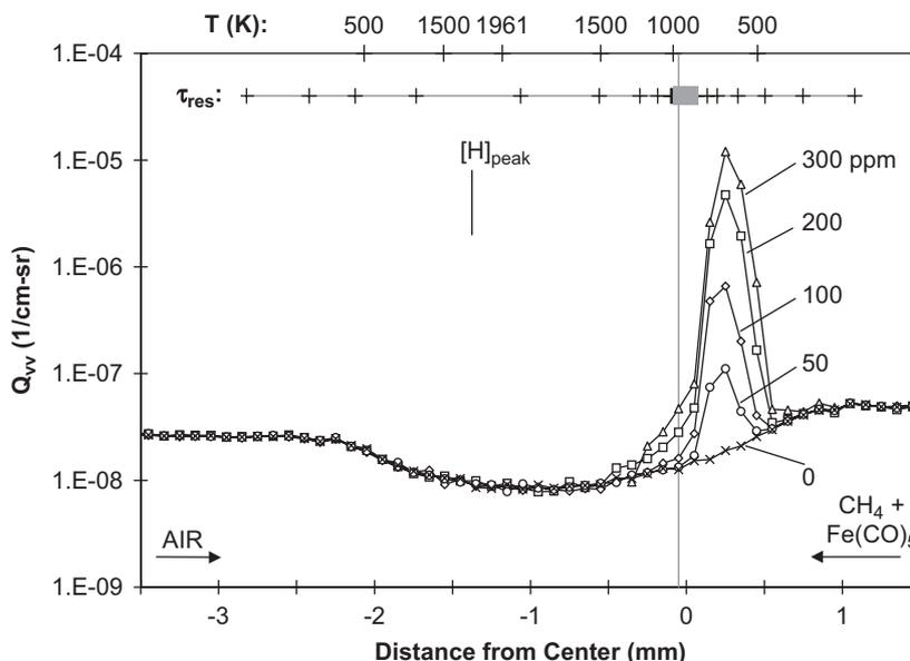
Fig. 30. Measured scattering profiles in  $\text{CH}_4$ -air counterflow diffusion flame with inhibitor in the fuel. The calculated temperature and point of peak H-atom mole fraction are marked on the upper x-axis, and the vertical line denotes the calculated location of the stagnation plane. Strain rate =  $330 \text{ s}^{-1}$  [45].
