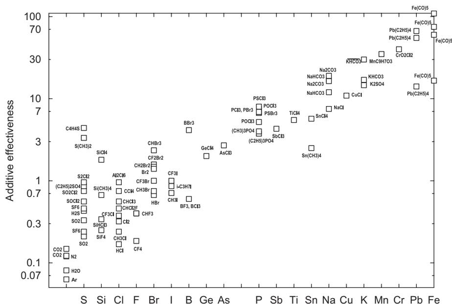
Fig. 2. Relative inhibitor effectiveness. Additive effectiveness is presented in coefficients of efficiency relative to  $\text{CF}_3\text{Br}$ . The compounds considered are mostly liquids or solids [78].
