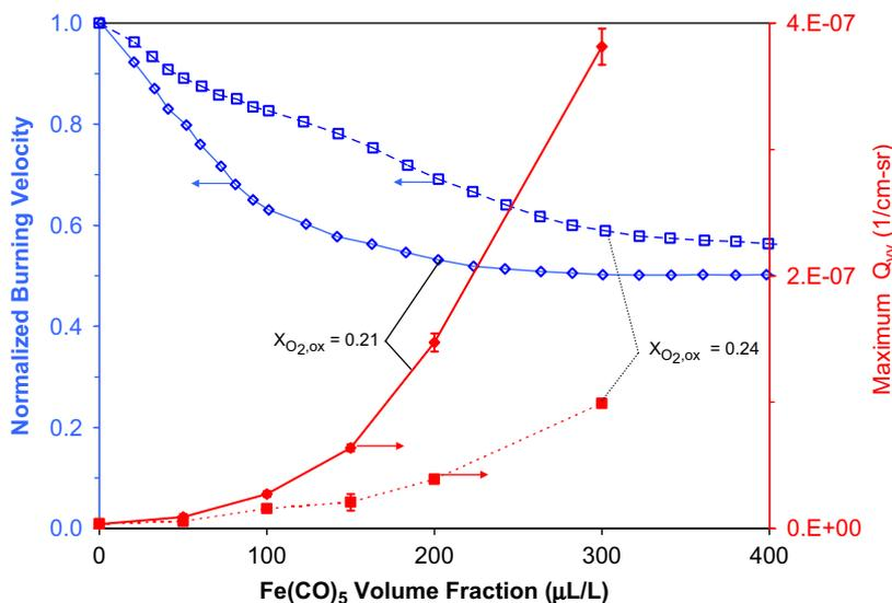
Fig. 24. Normalized burning velocity [9] and maximum  $Q_{vv}$  for  $\phi = 1.0$   $\text{CH}_4$  flame with  $X_{\text{O}_2,\text{ox}} = 0.21$  and 0.24 [41].
