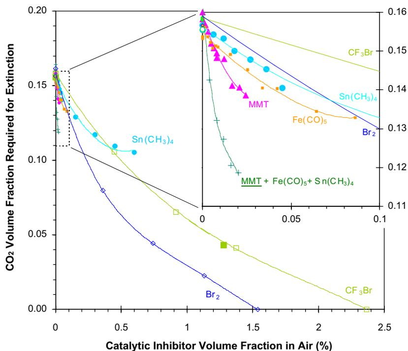
Fig. 34. Volume fraction of  $\text{CO}_2$  required for extinction ( $X_{\text{CO}_2,\text{ext}}$ ) of methane–air cup burner flames as a function of the volume fraction of catalytic inhibitor added to the air stream. Inset shows region in dotted box with expanded scales (points: experiments; lines: curve fits) [115].
