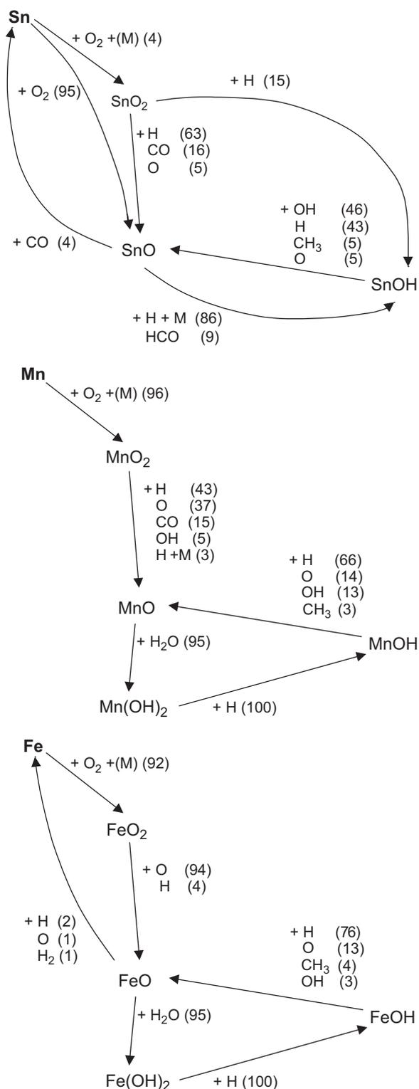
Fig. 19. Reaction pathways for Sn, Mn, and Fe in a premixed methane-air flame ( $\phi = 1.0$ ,  $X_{O_2,ox} = 0.21$ ,  $T_{in} = 353$  K). TMT, MMT, and  $Fe(CO)_5$  present at (1963, 128, or 105)  $\mu\text{L/L}$ , respectively. The numbers in parentheses are the fractional consumption (percent) of the reactant molecule.
