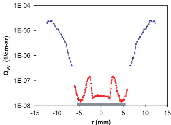
Fig. 22. Scattering cross section  $Q_{vv}$  as a function of the radial distance  $r$  from the burner centerline at 7 mm height in stoichiometric  $\text{CH}_4$ -air flame with  $200 \mu\text{L/L}$  of  $\text{Fe}(\text{CO})_5$  [41].
